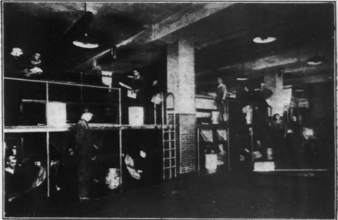
No acrobats need apply for press-climbing jobs here. All presses (below) are surrounded by the brass-railed wooden platform, the height of a man's chest from the floor. It's only a step from the tail of the plate-casting machine to the cylinders and the finished papers can be seen climbing through the ceiling to the mailing room and circulation department above. In the picture on the opposite page, the back-in platform where the auto-trucks and wagons load is seen in the new building in the background.
