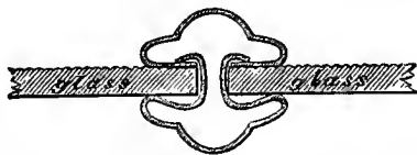
FIG. 63.—Section of Johnson's compressible glazing-tube.
