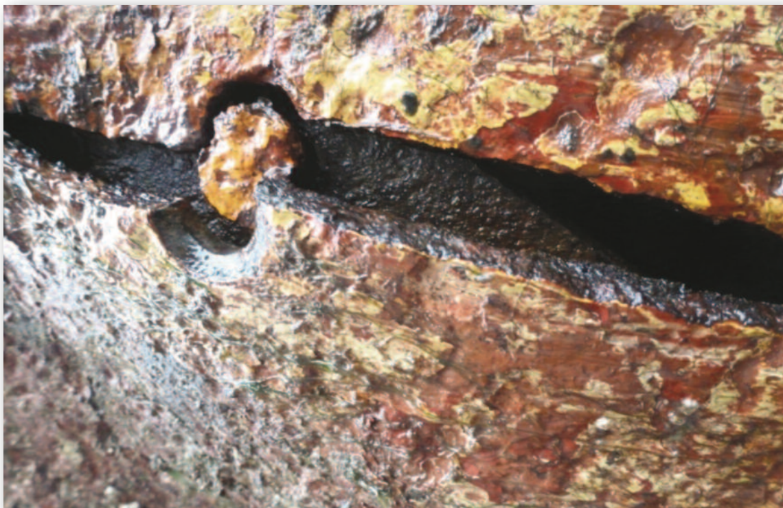
Photograph No.15 - Starboard side aft after salvage Note popped rivet
