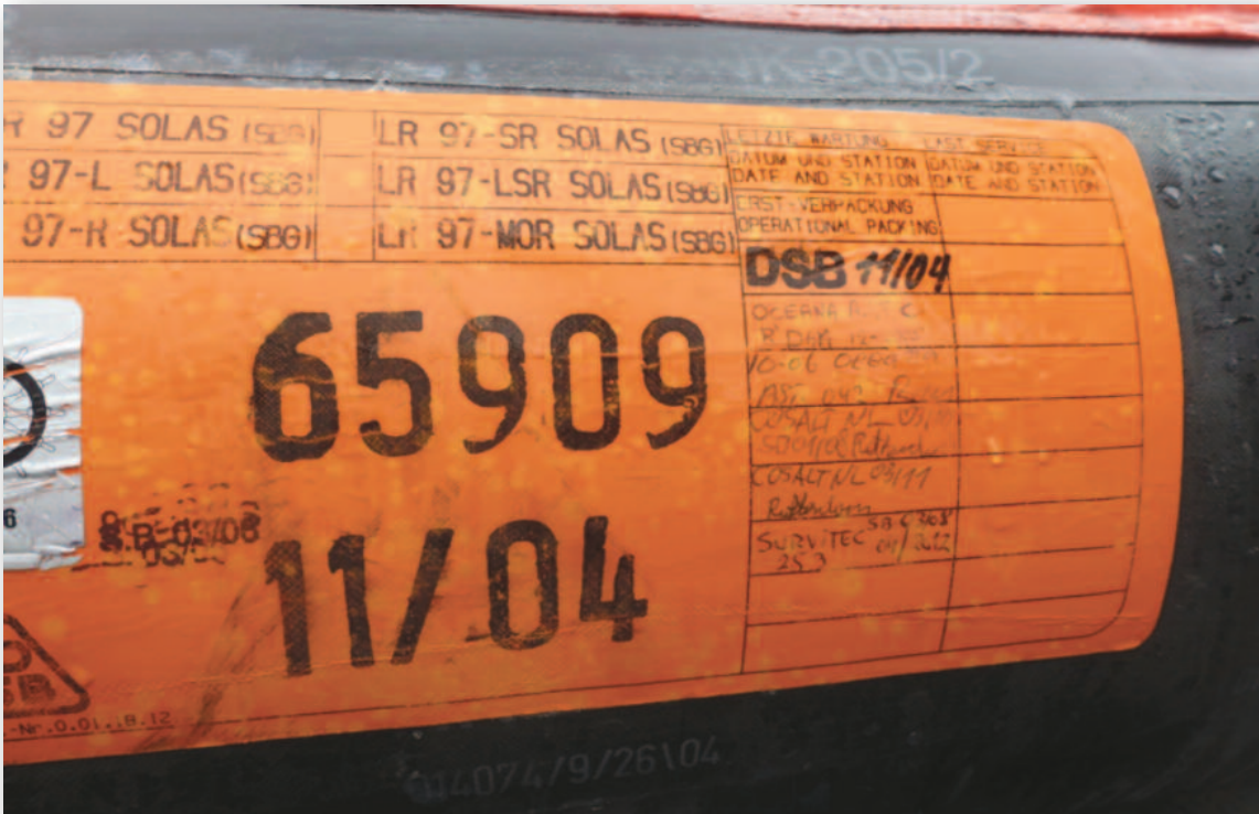
Photograph No.1 - Service label on liferaft showing annual survey not carried out
