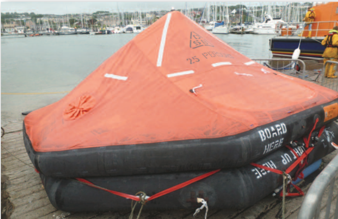
Photograph No.2 - Liferaft due service inflated as designed
