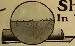
Edge of a dull razor— magnified.
