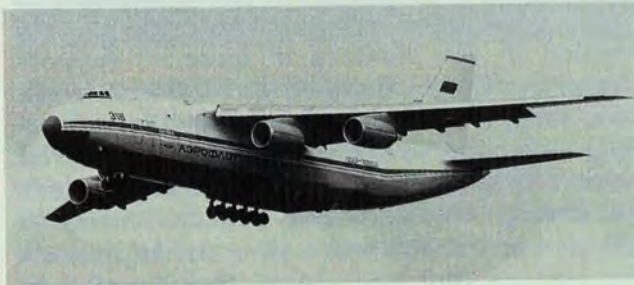
The An-124/CONDOR transport, which has a greater heavy-lift capability than the US C-5B Galaxy, may be deployed this year. CONDOR's visor nose and clamshell rear doors enable rapid drive-through loading and unloading.
