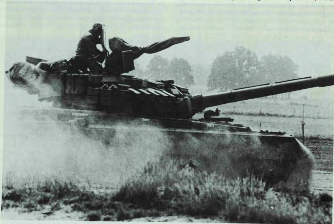
The box-like appendages around the turret of this T-80 tank are reactive armor. Exploding reactive armor dissipates the force of incoming antitank rounds, further protecting against the West's antitank capabilities.
