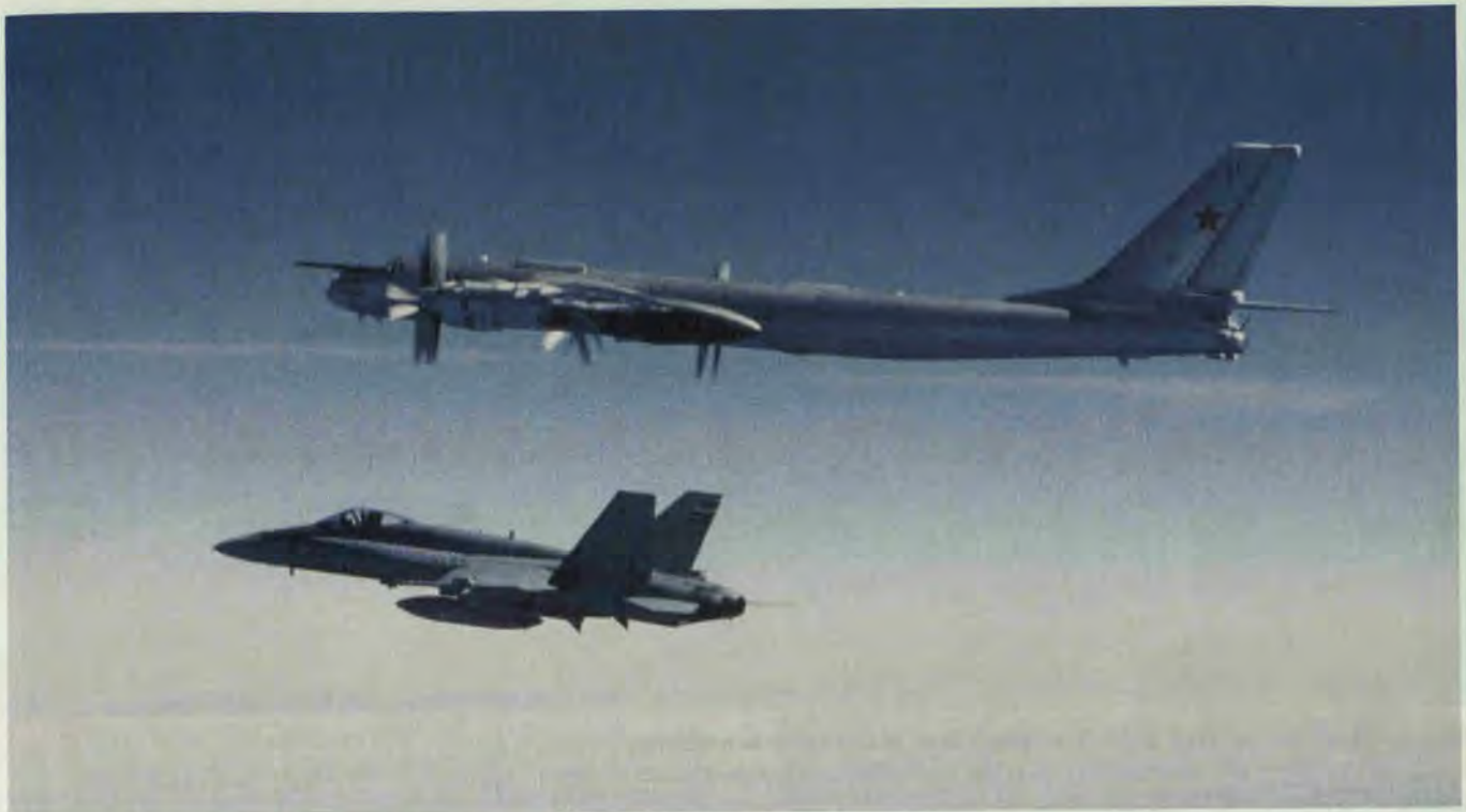
BEAR H bombers, which carry the 3,000-kilometer-range AS-15 cruise missile, have been intercepted by Canadian CF-18s while on training missions against North America.
