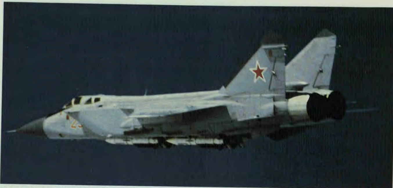
The MiG-31/FOXHOUND is one of the newest generations of supersonic interceptors with a look-down/shoot-down capability against aircraft penetrating at low altitudes.
