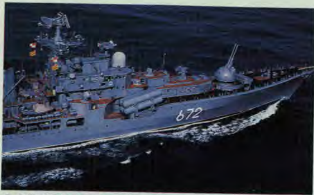
A SOVREMENNYY-Class guided-missile destroyer, with its forward twin 130-mm guns elevated, on its transit to the Soviet Pacific Fleet.
