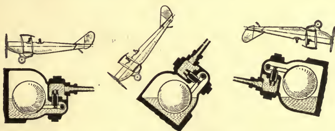
FIG. 209.—Diagram showing Stromberg float chamber in different orientations.
