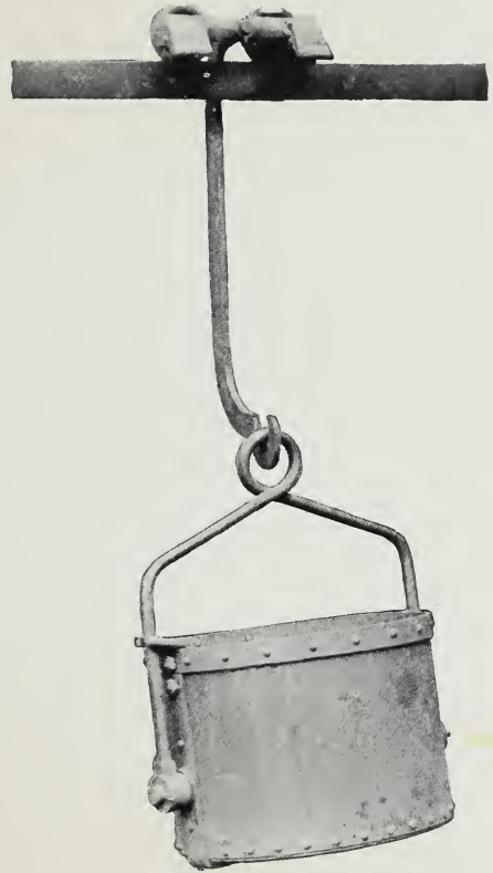
FIG. 61.—Bucket and Carrier (Endless Running Rope System).
