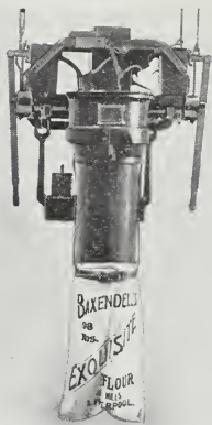
FIG. 91.—Simon's Dustless Sack Filling and Weighing Machine.
