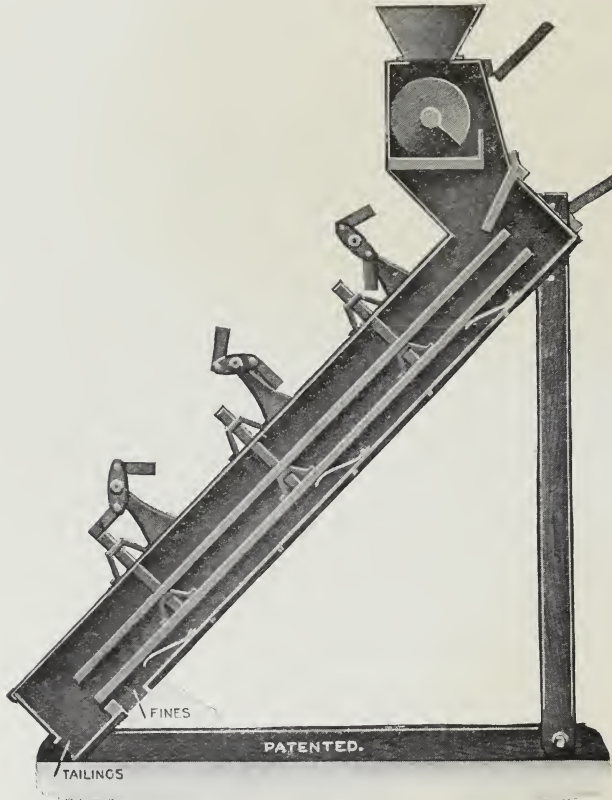
FIG. 96.—Section of Newaygo Separator with Guard Screen.
