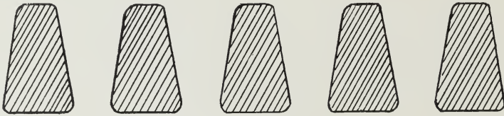
FIG. 3.—Section of Wash-Mill Grating.
