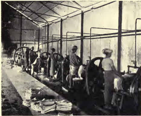
FIG. 56.—A Battery of Mills—Direct Drive (Bridge & Co.).
