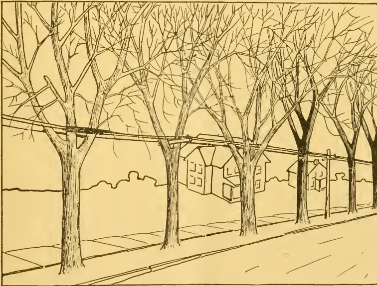
Fig. 13. The Same Trees as in Fig. 12, With Crowns Saved and Wires Carried Thru Them in Cables on Low Poles.
