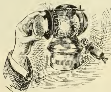
42—AN ACETYLENE LIGHT EGG TESTER
