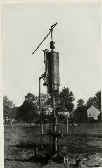
Fig. 52—Gas Pump for Pumping Water from Gas Well through \frac{3}{4} -inch Pipe, using the \frac{3}{4} -inch as a Sucker Rod and Tubing for Water Discharge Combined.
