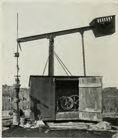
Fig. 55—Walking Beam Method of Pumping Water from a Gas Well. Power is furnished by 3 h. p. gas engine and the water is pumped through the \frac{3}{4} -inch siphon. The \frac{3}{4} -inch pipe is used as a sucker rod and tubing.
