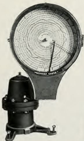
Fig. 135—Mercury Float Recording Differential and Static Pressure Gauge. This gauge carries two pen arms marking on one chart
