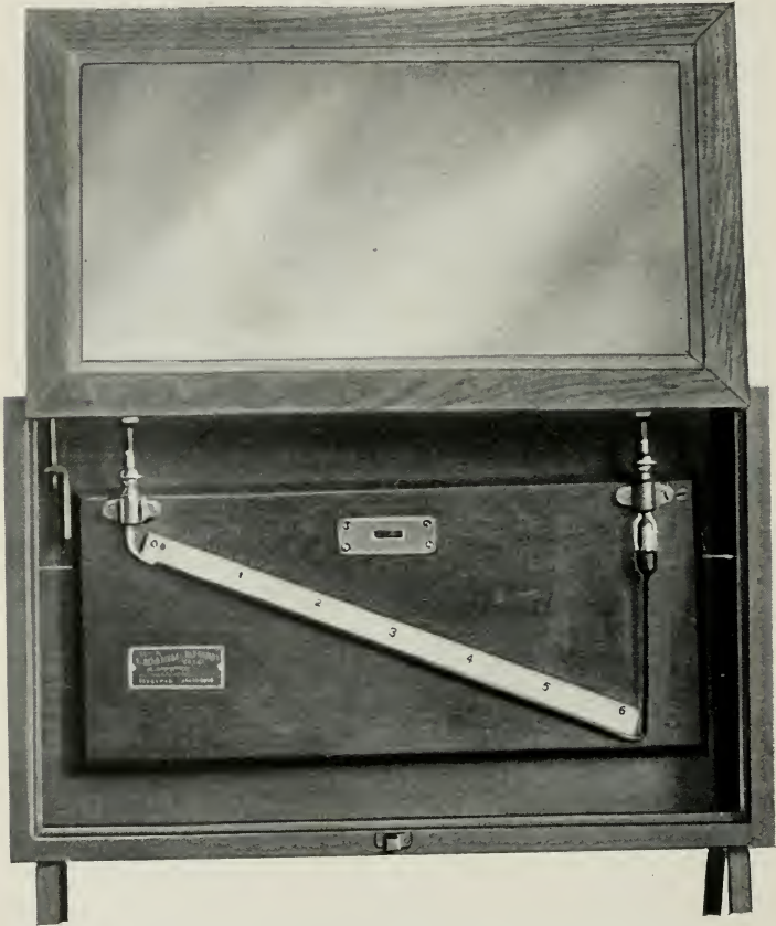
Fig. 144—LOW PRESSURE GAUGE Used in proving Large Capacity Meters. Can be used as a Differential Gauge, also for proving Domestic Meters
