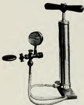
Fig. 179—GAS PROVING PUMP AND GAUGE
