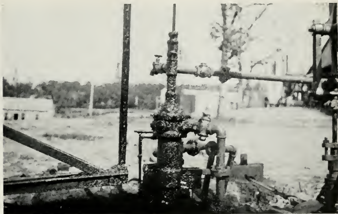
Fig. 220—A PUMPING OIL WELL SHOWING "CASING HEAD" AND LEAD LINES TO CARRY THE GASOLINE GAS TO THE COMPRESSING PLANT
