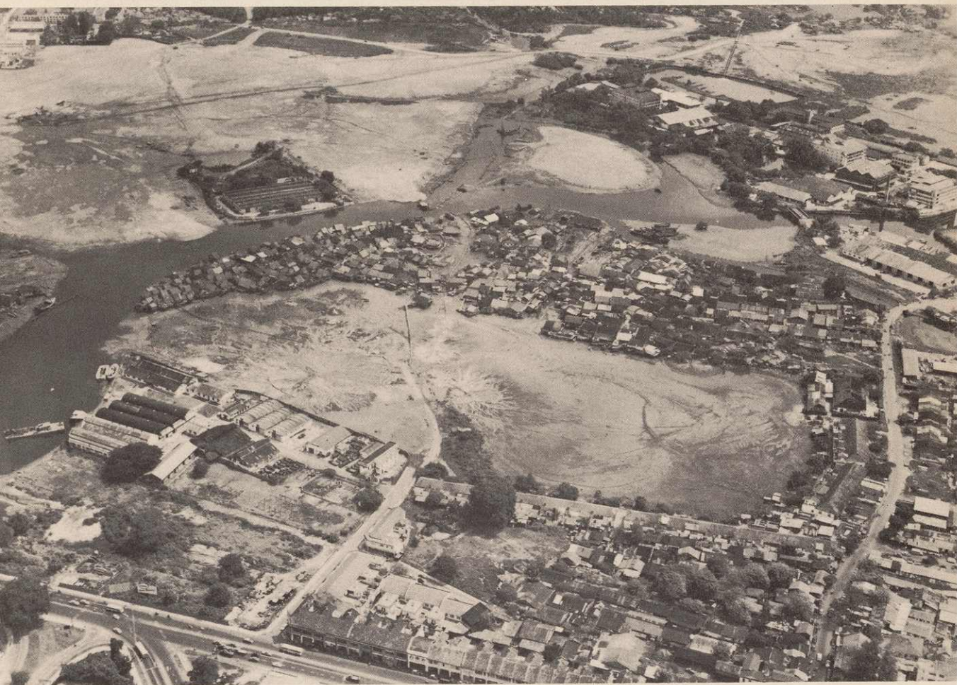
Aerial view of the reclamation work in progress at Kallang Basin (230 acres of swamp land have been reclaimed by the end of 1966.)
