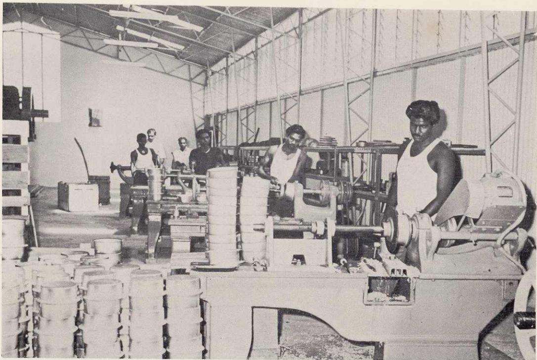
Tanglin Halt Industrial Estate: Aluminium holloware factory—manufacture of aluminium cooking utensils.
