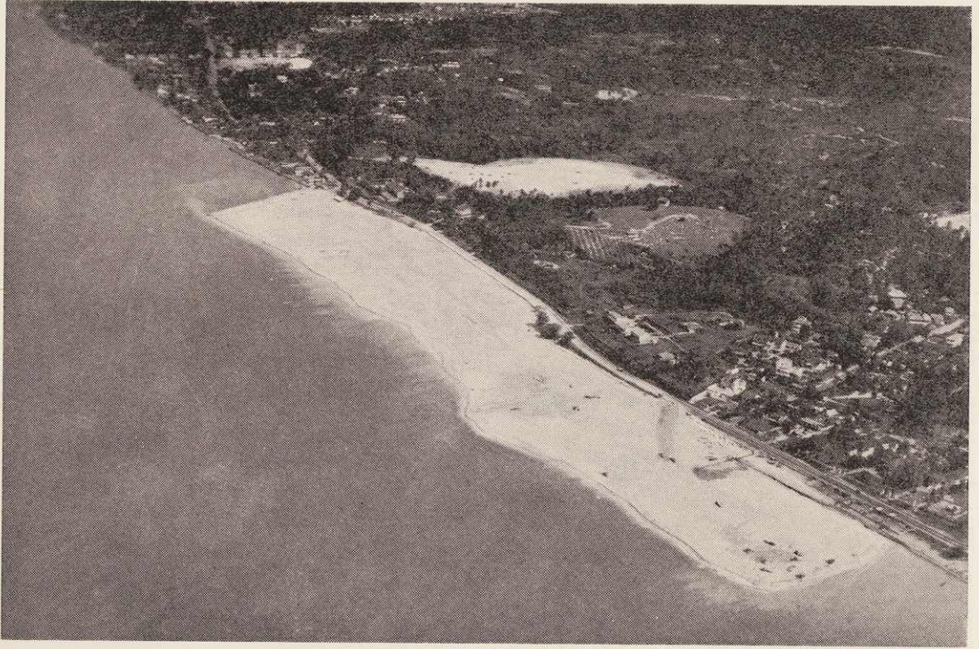
Aerial view of the 48 acres reclaimed at Bedok under the Board's pilot scheme.
