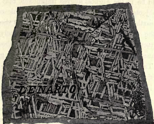
Fig. 38.—Slab of Crystallised Iron cut from the Aerolite of Lenarto, Hungary.
