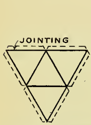
Fig. 500.—Development of tetrahedron.
