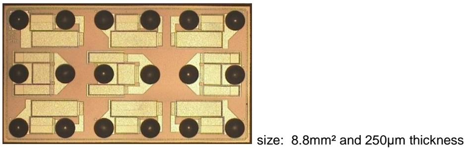
Figure 10: The Silicon Capacitor array with PICS1
