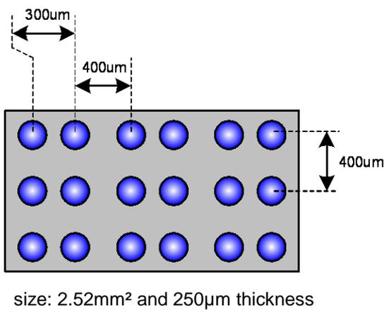
Figure 11: The Silicon Capacitor array with PICS2
