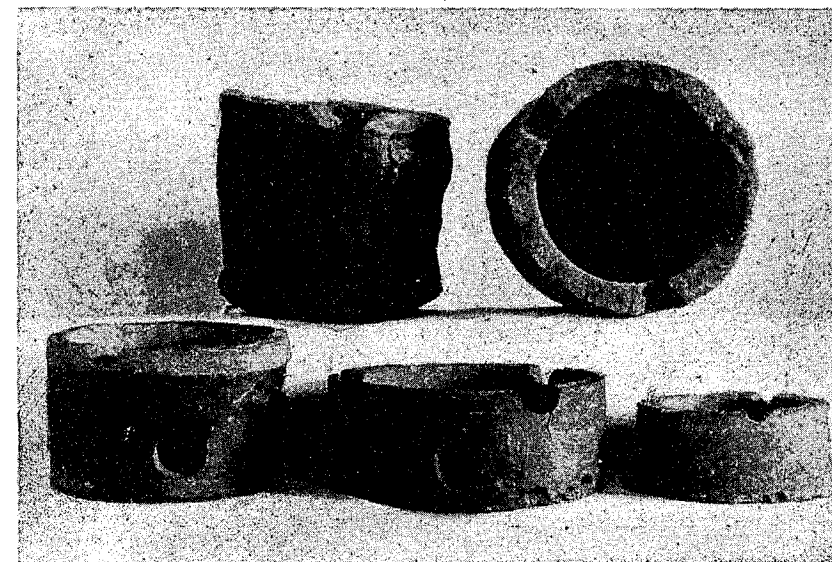
2. Saggars in which porcelain bowls and dishes were baked in the Liu Li Ch'ang and the Ch'ung Lai kilns. In the saggars the dishes were protected from the intense heat.
