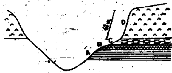
Fig. 3. Section behind Yisukan 依斯坎後剖面圖: A, Black shale with coal seam 黑頁岩夾煤層; B, White sandstone 白砂岩; C, Green and grey tuff 綠及灰色凝灰岩; D, Andesite 安山岩。
