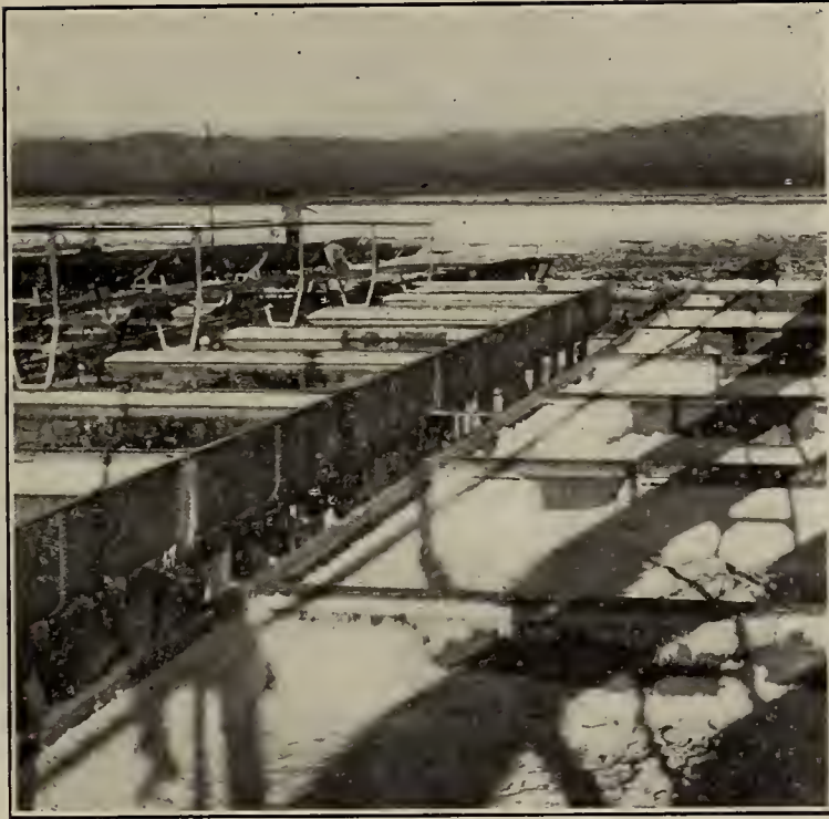
The crystallizing tanks. Refined nitrate in the tanks in the foreground; tanks recently filled with caldo in the background.
