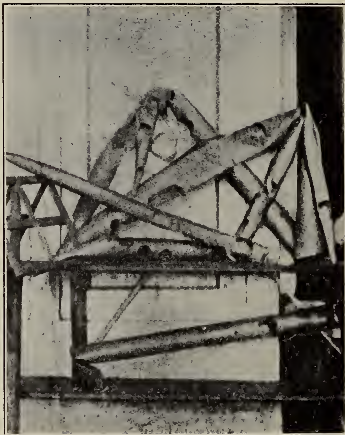
FIG. 8. ORGAN PIPES THAT HAVE BEEN ATTACKED BY THE TIN DISEASE.
