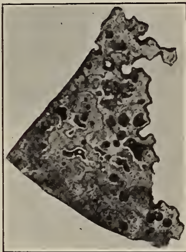
FIG. 9. THE SPREAD OF THE TIN DISEASE ON A PIECE OF SHEET TIN.
