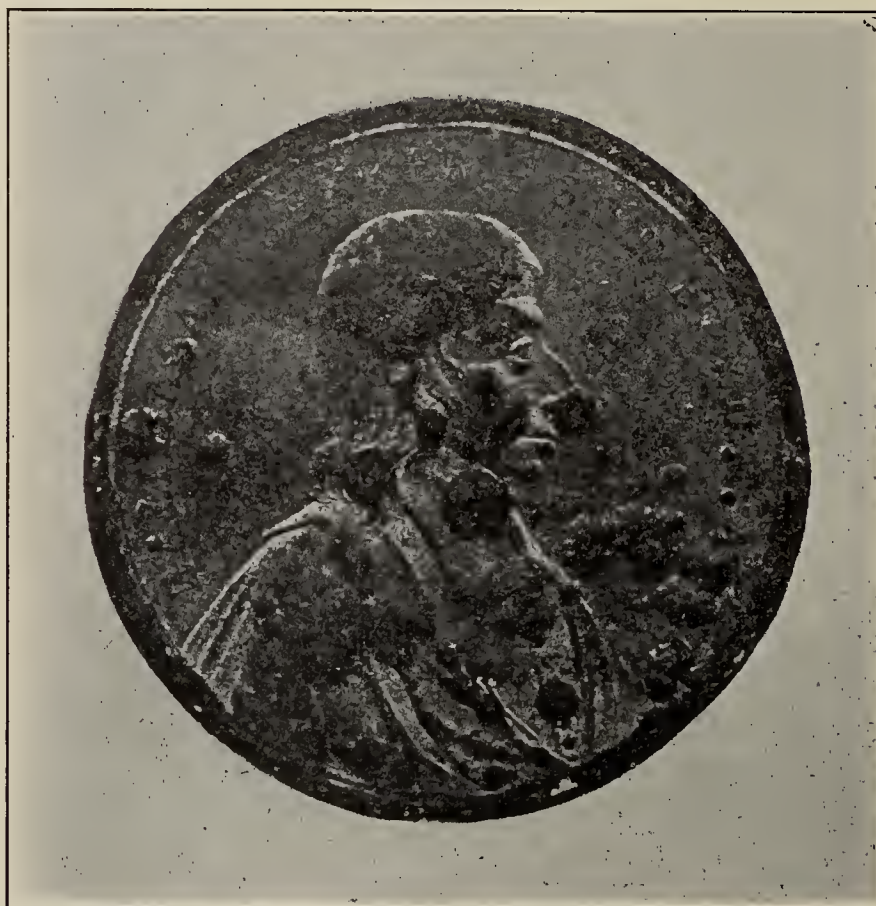
FIG. 10. A TWO-HUNDRED-YEAR-OLD MEDAL THAT IS SUFFERING FROM THE TIN DISEASE.
