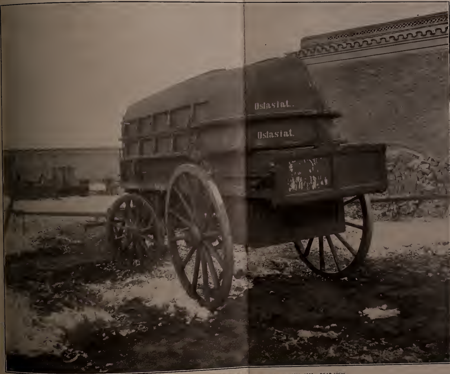
171 GERMAN PONTON WAGON CARRYING TWO HALF BOATS (ADVANCE GUARD), TIENSIN, 1900. REAR VIEW.
