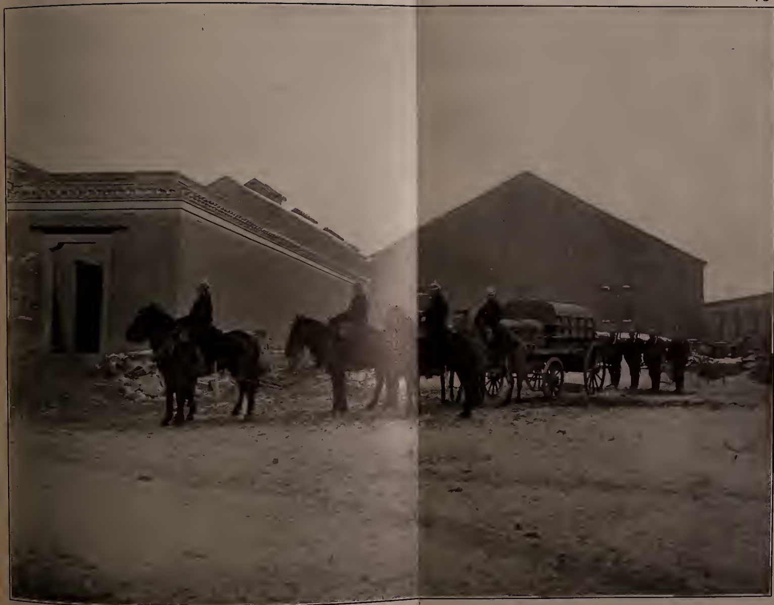
GERMAN PONTON WAGON CARRYING TWO HALF BOATS (ADVANCE GUARD), TIENSIN, 1900. FRONT VIEW.
