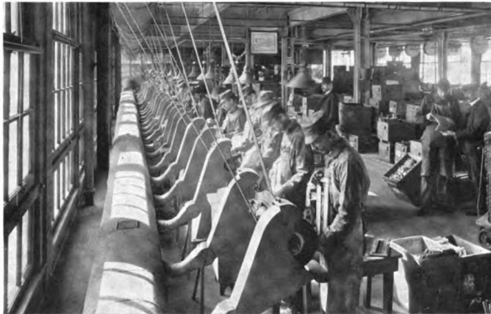
The polishing room is kept clean and healthful by an exhaust system which carries away the metal dust.
