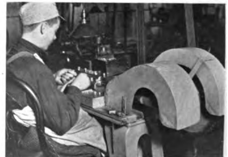
Guards over gears on thread rolling machine.
