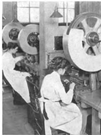
Gears are protected by metal guards.
