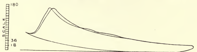
Nominal HP, 6; diam. of cylinder, 9\frac{1}{8} " ; length of stroke, 16" ; rev. per min. 180; consumpt. per IHP hour, 15.03 cb. ft. ; consumpt. per BHP hour, 20.808 cb. ft. ; scale of spring, \frac{1}{180} " per lb. ; max. pressure, 171 lbs. ; pressure before ignition, 69 lbs.
