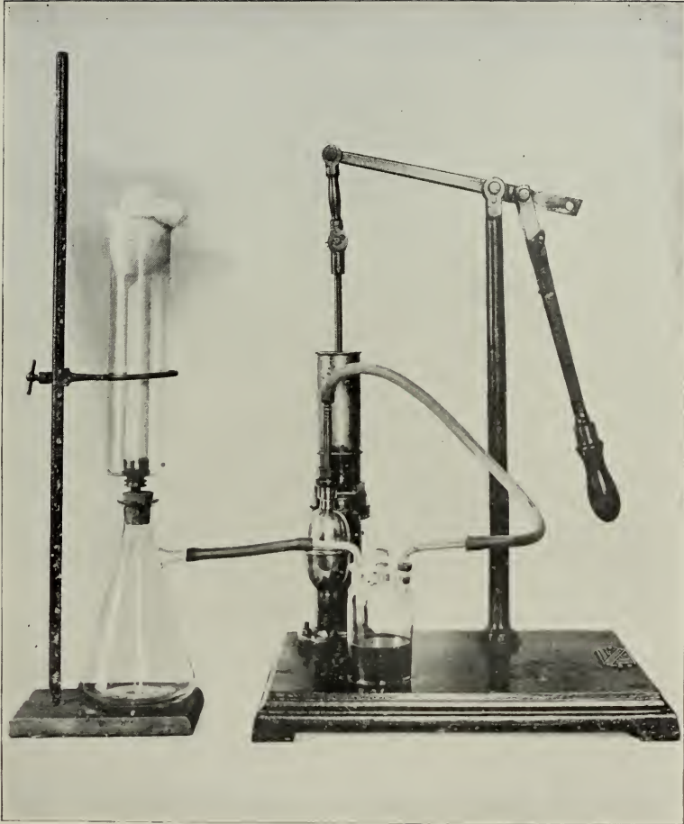
APPARATUS FOR FILTERING WATER TO FACILITATE ITS BACTERIOLOGICAL EXAMINATION. (The filter-brushing method).
