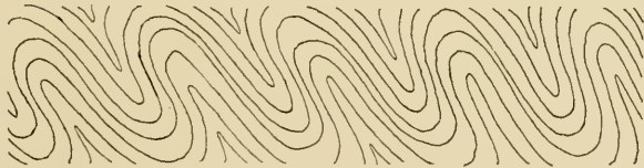
FIG. 5.—Diagram showing type of unsymmetrical overturned folding.
