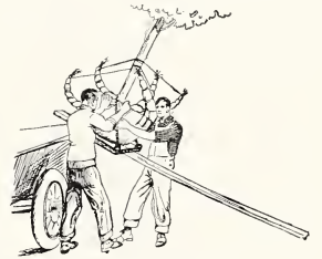
Tree is loaded on a truck by roller skids and laid down to go under wires. It is unloaded by standing it up and sliding it off on your grounds. It may weigh five or ten tons. The Hicks tree-moving crews handle it as easily as a safe is put into a bank.
