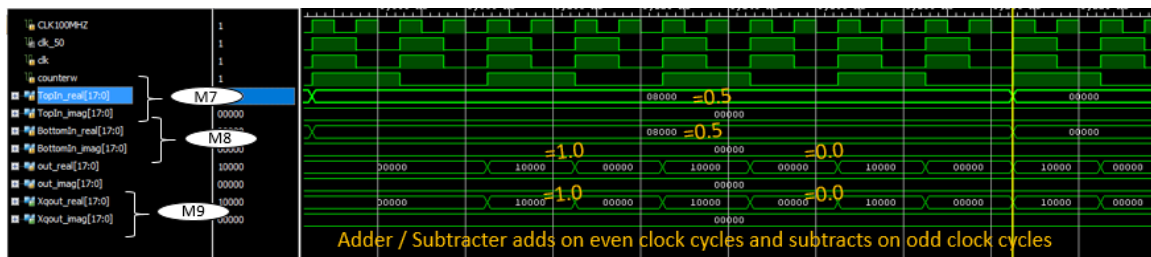
Figure 56. Adder / Subtractor Adds on Even Clock-Cycles
