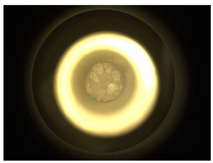
NASA's Perseverance Mars rover took this image of regolith – broken rock and dust – on Dec. 2, 2022. This regolith, contained inside a metal tube, is one of two samples that will be considered for deposit on the Martian surface as part of the Mars Sample Return campaign.
