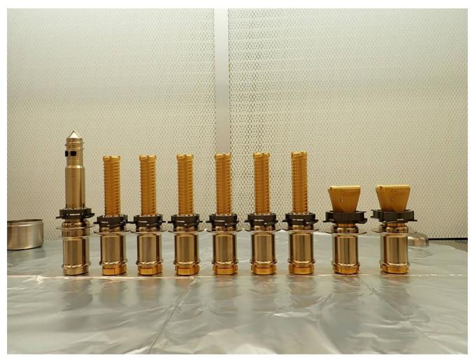
The drill bits used by NASA's Perseverance rover are seen before being installed prior to launch. From left, the regolith bit, six bits used for drilling rock cores, and two abrasion bits used to remove the dust-covered outer layer of a rock so that the rover can take accurate data of its composition.
