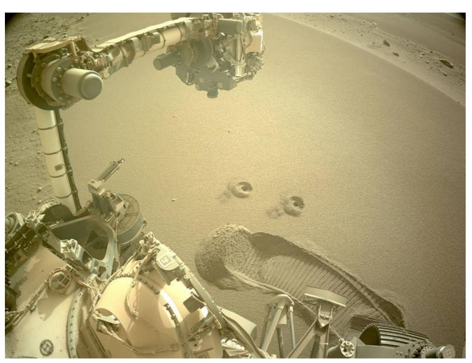
Two holes are left in the Martian surface after NASA's Perseverance rover used a specialized drill bit to collect the mission's first samples of regolith - broken rock and dust - on Dec. 2 and 6.
