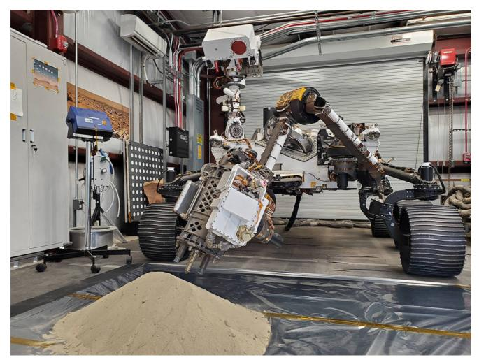
Optimism, a full-scale replica of NASA's Perseverance Mars rover, tests a model of Perseverance's regolith bit in a pile of simulated regolith – broken rock and dust – at JPL.
