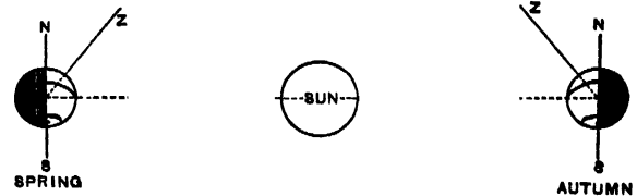
FIG. 45.—Diagram showing the equality of the sun's zenith distance at the two equinoxes. N, north pole of the earth; S, south pole; Z, zenith of Greenwich.
