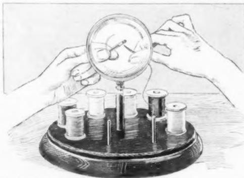
Magnifying Glass Mounted on Sewing Machine Relieves Eye Strain When Threading Needles
