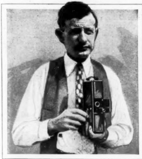
Compact Camera Which Uses Standard-Size Motion-Picture Film to Take 400 Exposures
