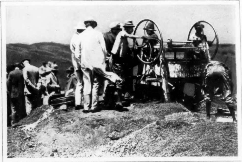
The "Baby" Washing Machine Cleaning Gravel in Search of Diamonds beside a Stream Bed at Mafeking; Diamond Mining Is Much Simpler Than Taking Minerals from Ore
