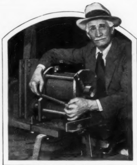
Part of the Outfit for Making Hollow Steel Axles and Other Units in Faster Time
