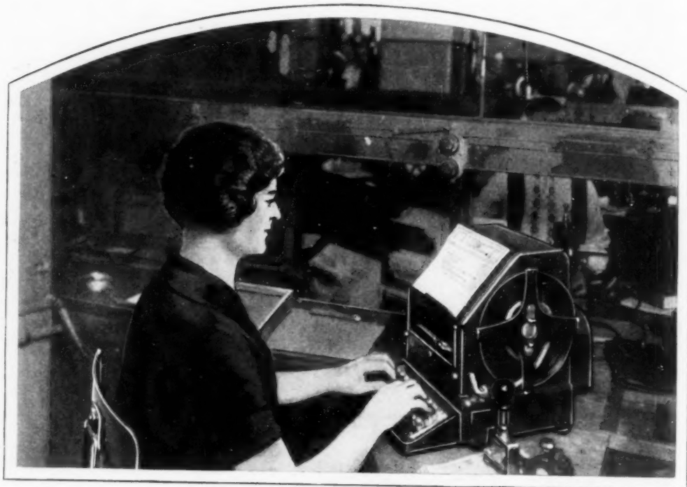
The Automatic Printing Telegraph, Operated from a Typewriter Keyboard, Is Typical of Inventions That Have Won Their Owners Both Fame and Fortune
