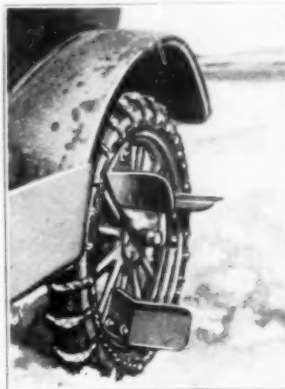
Sheet-Metal Snowshoes on Rear Wheels Help Auto Travel in Deep Snow
