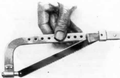
Method of Using a Broken Hacksaw Blade
