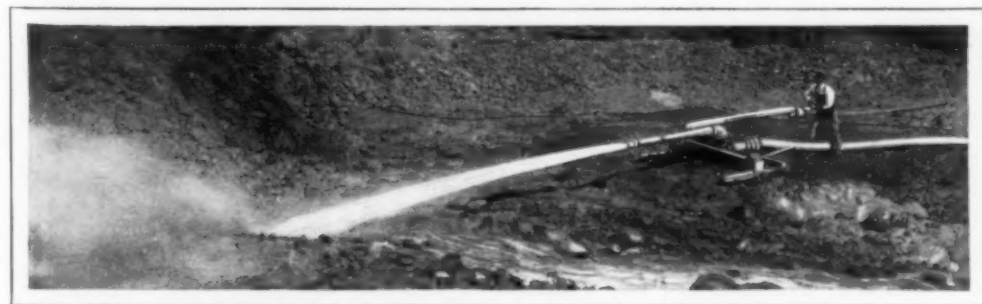
Compare This with the Patient Panner Above; the Hydraulic Gun of the Placer Diggings Washes Whole Hillside into the Sluice Boxes under the Force of Tremendous Pressure
