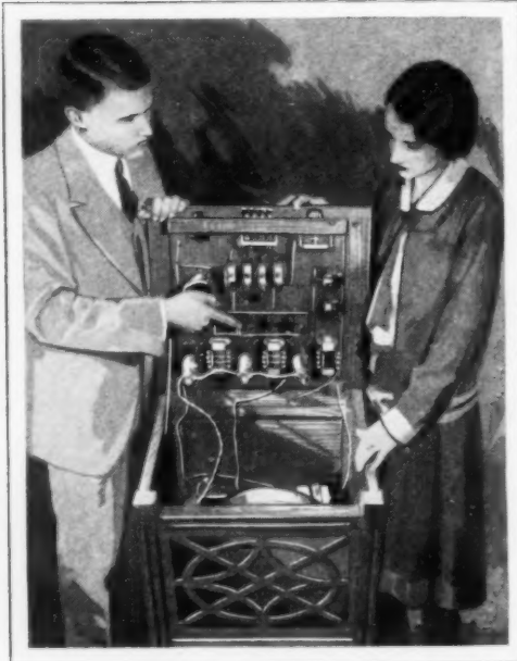
What the Subscriber Doesn't See in the Sealed Cabinet: a Complete Three-Tube Radio Set
