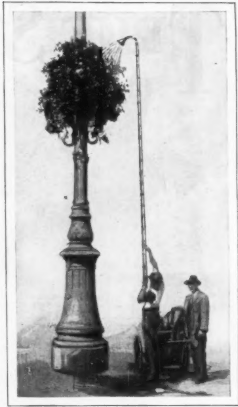
Sparing the Attendant a Climb up a Ladder; Watering Street Pole Garden with Extension Sprinkler
