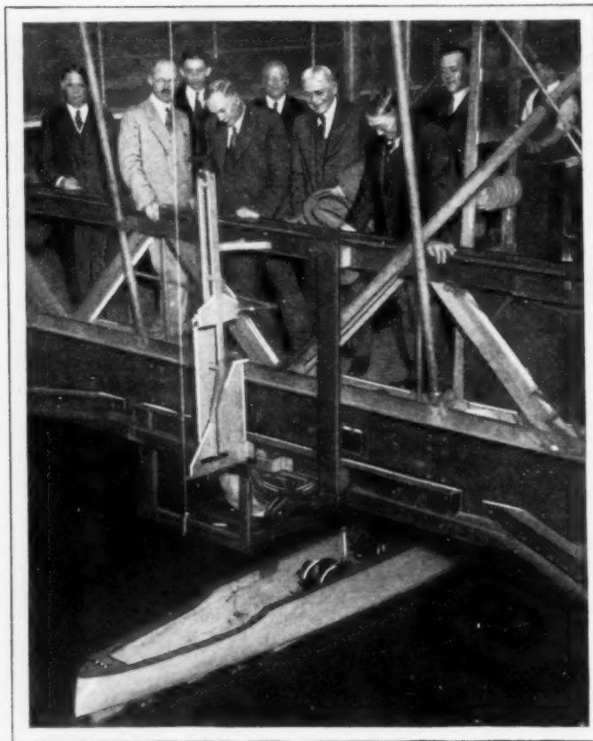
Officials Watching from the Crane Bridge as Model of Transatlantic Hull Is Tested in Towing Basin
