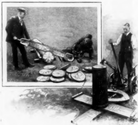
Demonstrating the Wire Band Saw and the Hand-Operated Saw for Felling Trees
