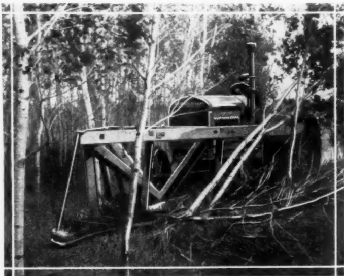
Mowing Down Trees with a Tractor: a Cutter Attachment in Front Slices Off the Brush and Small Growth
