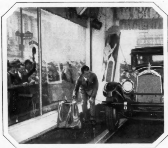
By Passing His Hand over the Opening in the Window, the Man Outside Is Able to Start Demonstration Auto through Action of Relays
