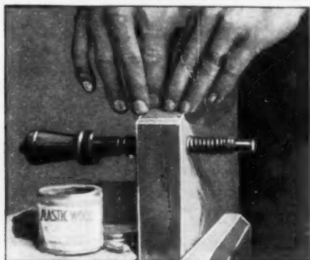
Forming the Nut in Mold by the Use of Plastic Wood
