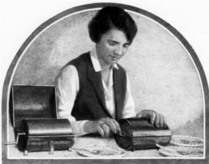
Preparing Ice Cream at the Table; the Freezer Is Shown Open at the Left and in Operation at the Right
