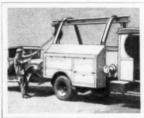
Wrecking Truck with Supply Cabinets Built Out over the Fenders of the Car
