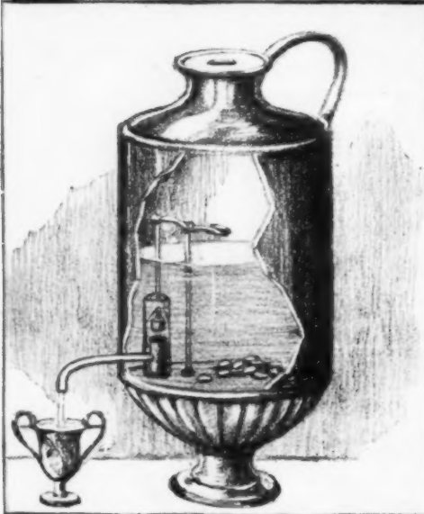
Slot Machine Dispensing Temple Water to Worshipers, and, Above, Statues That Poured Magic Libations
