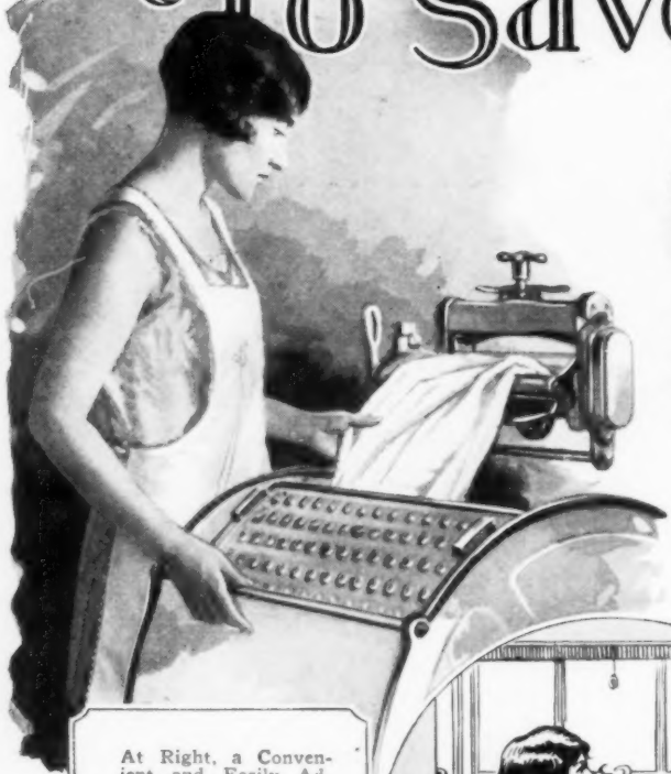
To Keep the Fingers Away from the Wringer, the Washing Machine at Left Is Fitted with an Automatic Feeding Attachment; Above, an All-Rubber Dish Scraper That Won't Break, and Saves the Plates
