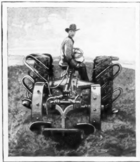
Giving the Tractor Added Efficiency; Wheels Equipped with Special Lugs for Soft Soil
