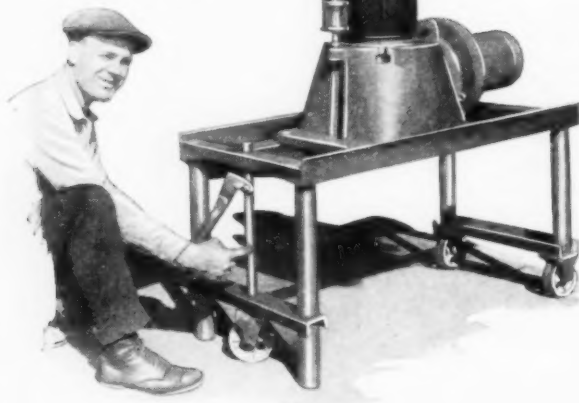
Convenient Truck Which May Be Made Stationary by Lowering the Legs
