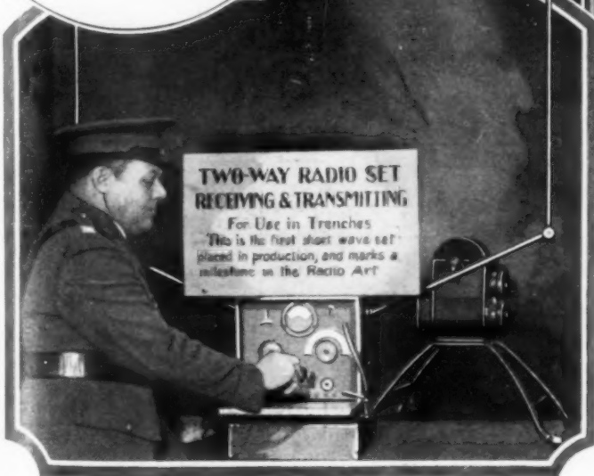
Left, Captain Autrey, of the U. S. Signal Corps, with One of the Latest Types of Radio-Receiving and Transmitting Sets Designed for Use in Trenches; These Two-Way Short-Wave Sets Are Portable and Mark an Advanced Step in Radio Communication as Applied to Field Use under War Conditions
