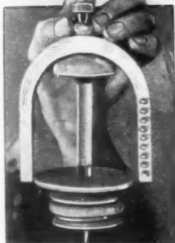
Assembly of Flier, Pulley and Spindle Eye
