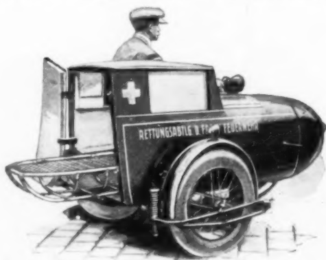
© Henry Miller Motorcycle Sidecar Ambulance for Emergency Service in the Berlin Fire Department
