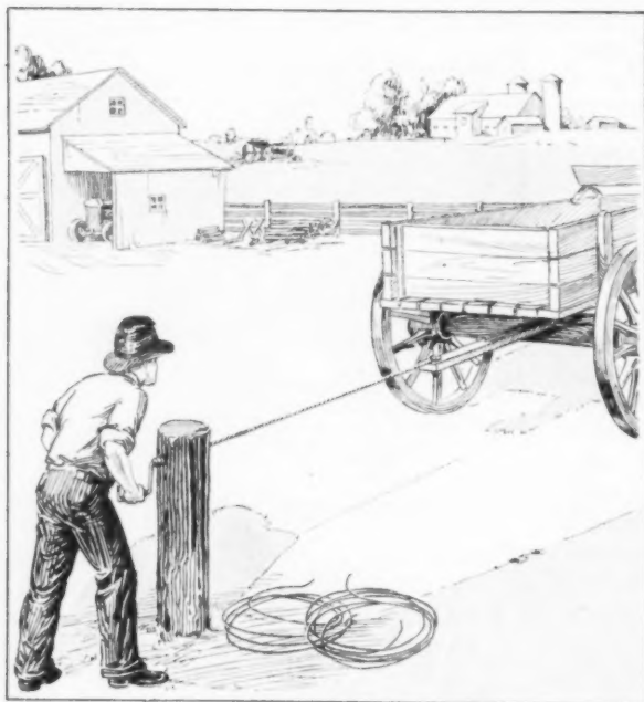
Quick and Easy Method, Used by Wisconsin Farmer, of Twisting Four Wires into a Strong Cable
