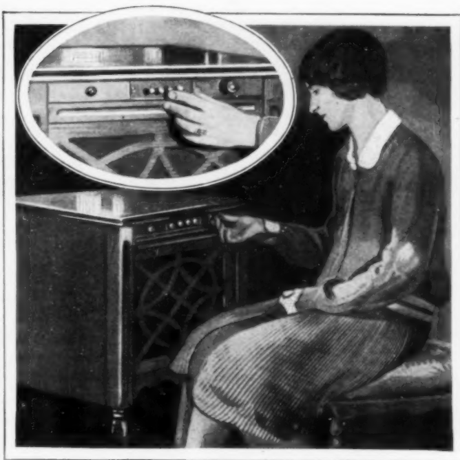
The Radio Receiver and Loud Speaker, and, Inset in Oval, a Close-Up of the Four Push Buttons, Switch and Volume Control
