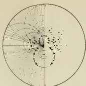
Fig. 2 Stereographical Projection of the Röntgenogram of Turmaline. Plate parallel to (0110) .
