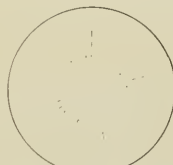
Fig. 14 Stereographical Projection of the Röntgenogram of dehydratory Quartz. Plate parallel to (0001) .
