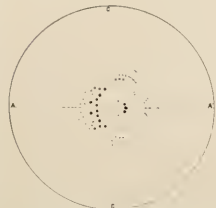
Fig. 16. Stereographical (Schematic) Projection of the Röntgenogram of Zinc sulphate. Plate parallel to (010). Abnormal Pattern, obtained with a perfectly clean lamella prepared by cleavage, and exactly perpendicular to the first bisectrix.
