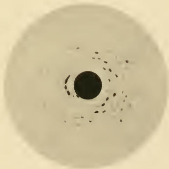
Fig. 17. Zinc-Sulphate Cleavage-lamella, exactly parallel to (010). (The b -axis is 1 st bissectrix).
