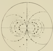
Fig. 6 Stereographical Projection of the Röntgenogram of Dolomite. Plate parallel to (1110) .
