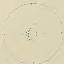
Fig. 26. Stereographical Projection (schematic) of the Röntgenogram of Zinc-sulphate. Plate parallel to (1010). (Abnormal image, obtained with a perfectly clear lamella, prepared by cleavage, and exactly perpendicular to the first bisectrix).
