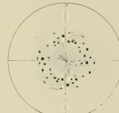
Fig. 8 Stereographical Projection of the Röntgenogram of Calcite. Plate parallel to (1110) .
