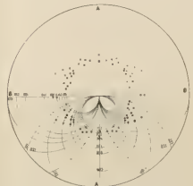
Fig. 19. Stereographical Projection of the Röntgenogram of Isogyrate Asparagine. Plate parallel to (001) (Schematic).
