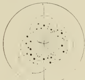
Fig. 5 Stereographical Projection of the Röntgenogram of Dolomite. Plate parallel to (0110) .
