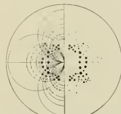
Fig. 11 Stereographical Projection of the Röntgenogram of Beryl. Plate parallel to (1110) .
