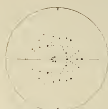
Fig. 18. Stereographical Projection of the Röntgenogram of Nepheline. Plate parallel to (1210).
