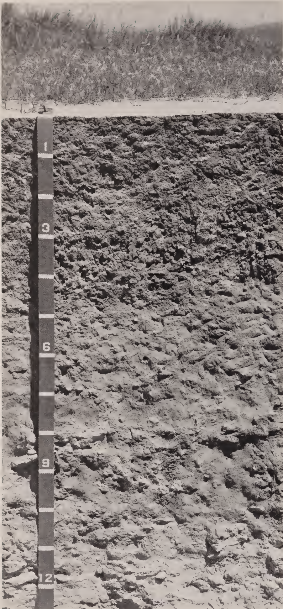
Figure 13.—Profile of Sebree very fine sandy loam in an area of Purdam-Sebree-Owsel complex, 0 to 8 percent slopes (numerals on tape indicate decimeters). A silty clay layer that has a high sodium content is just below the surface, and a hardpan is at a depth of about 32 inches (8 decimeters).
