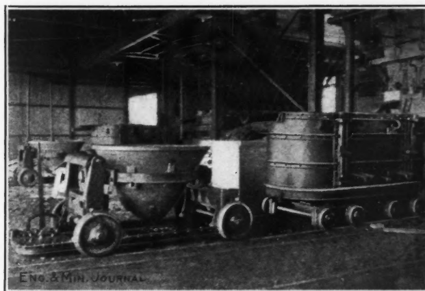
FIG. 3. FOREHEARTH AND SLAG POT
