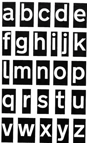
Fig. 2. Transport Medium lower-case alphabet for use on signs with dark backgrounds. (Paragraphs 44 and 141 and Appendix VIII.)
