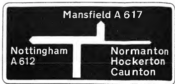
Fig. 84. Advance direction sign for staggered junction. (Paragraph 148.)
