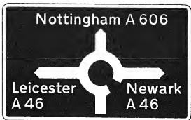
Fig. 80. Advance direction sign for roundabout junction. (Paragraph 148.)
