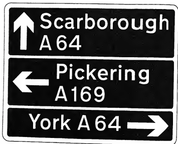
Fig. 85. Stack type advance direction sign. (Paragraph 148.)
