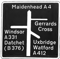
Fig. 78. Advance direction sign for complex junction. The relative importance of each road is shown by differing the width of the route symbol. (Paragraphs 144, 148 and 150.)
