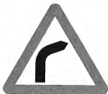
Fig. 37. Bend to the right. (Paragraph 91.) (The symbol may be reversed.)
