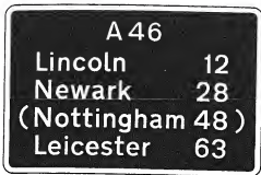
Fig. 93. Route confirmatory sign. (Paragraphs 154 and 280.)
