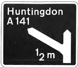
Fig. 76. Advance direction sign for use \frac{1}{2} mile before grade-separated junction. (Paragraphs 148 and 280.)
