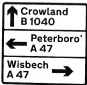
Fig. 88. Stack type advance direction sign for non-Primary routes. (Paragraph 148.)
