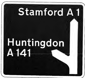
Fig. 77. Advance direction sign for use at beginning of deceleration lane at grade-separated junction. (Paragraphs 148 and 280.)
