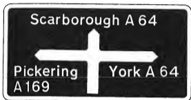
Fig. 74. Advance direction sign for simple cross roads. (Paragraph 148.)
