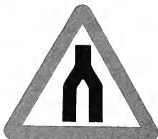
Fig. 42. Dual carriageway ends. (Paragraph 111.)
