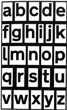
Fig. 5. Transport Heavy lower-case alphabet for use on signs with white backgrounds. (Paragraphs 44 and 141 and Appendix VIII.)
