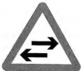
Fig. 44. Two-way traffic across a one-way carriageway. (Paragraph 111.)
