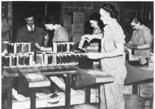
Mr. Benjamin P. W. Ruotolo samples air for lead at battery plate separating operation.
