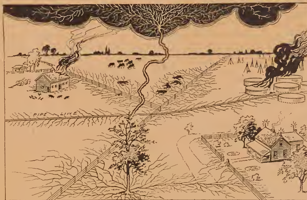
This visualizes in a graphic manner the discharge of the earth's "electrical field." It shows graphically the reason for greater electrical intensity on the earth's surface, around the tree, along the wire fence and the oil pipe line, than elsewhere and why a lightning flash occurs. Cattle are struck dead near a wire fence, while other cattle out in a field are not affected. Petroleum tanks adjacent to the pipe line are ignited. An unprotected barn is in flames; but the dwelling, properly rodded, is immune.
