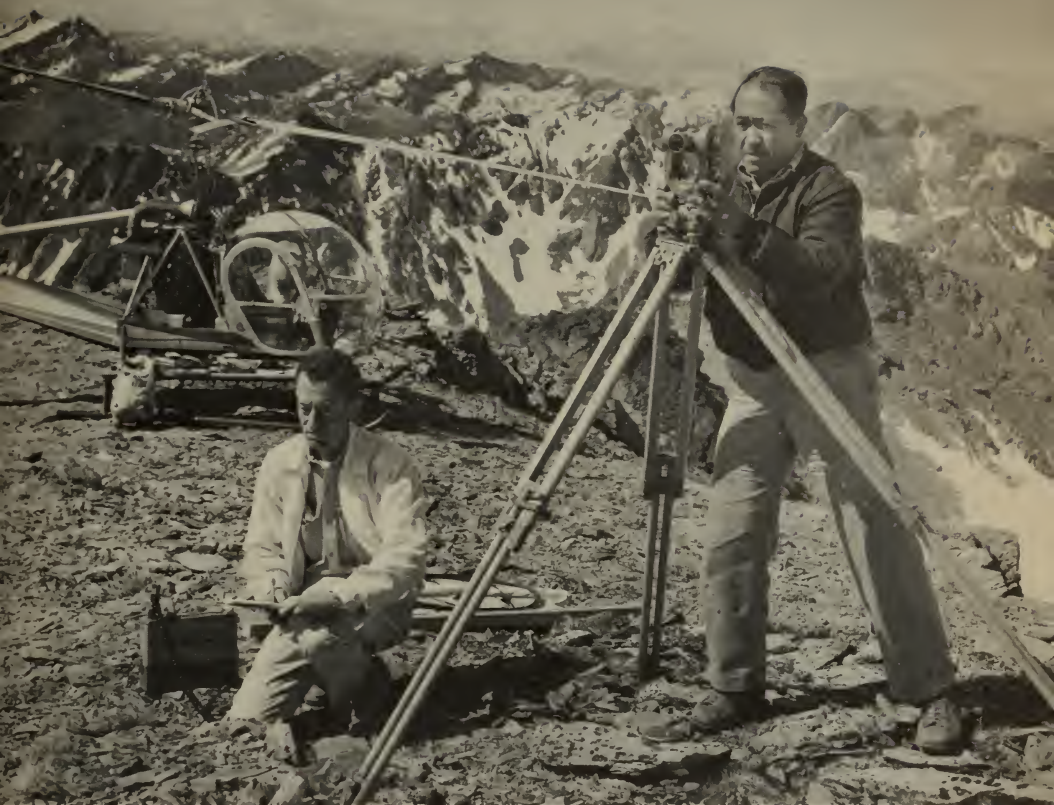
Control surveys for topographic mapping in rugged western mountains employ helicopters and two-way shortwave radio.
