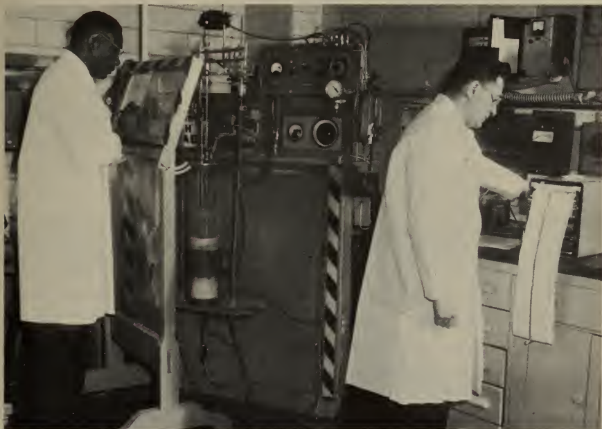
In the tall, cylindrical cell a protective coating of molybdenum metal is being electro-deposited at 900^{\circ} C. Guarded by a safety screen against accidental exposure to the high temperature, a Bureau of Mines scientist takes notes while another checks a recording device.
