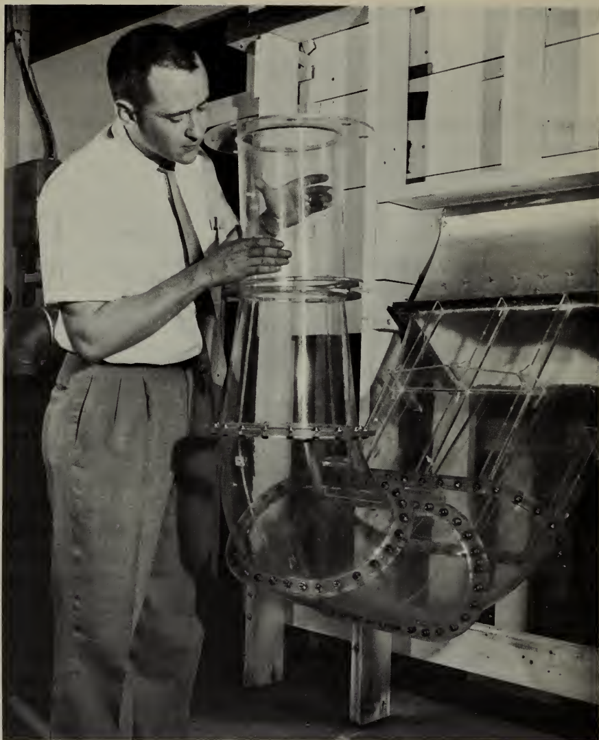
A hydraulic engineer in the Bureau of Reclamation's research laboratories in Denver, Colo., checks the model of the new improved suction inlet tube developed for use in large pumping plants.
