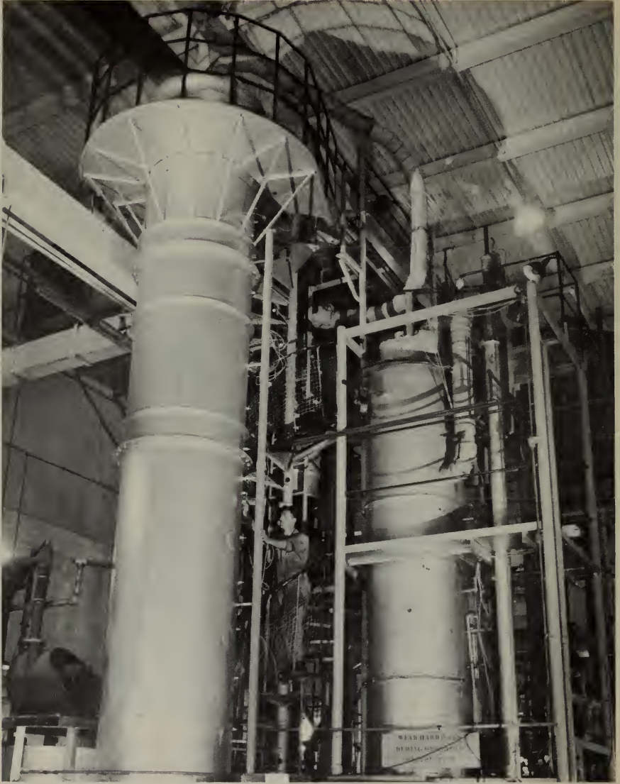
Valuable products, including chemicals and cokelike fuels, have been made from high moisture coal in the Bureau of Mines carbonizing reactor to the left. Costs are low, and the process holds promise of opening new markets for coals that would otherwise be more limited in their usefulness.
