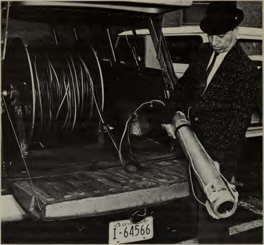
This small diameter TV camera is used for subsurface geologic and hydrologic exploration.
