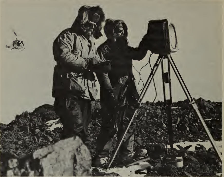
Survey engineers in a helicopter supported geodetic traverse in Antarctica using electronic equipment to measure the distance to a companion unit on a distant mountain peak.
