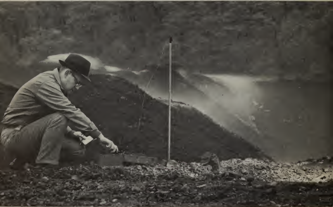
A Bureau of Mines engineer measures the combustion rate of a smoldering coal refuse pile during studies on how to control such sources of air pollution. Vapors in the background show clearly in this photograph but most atmospheric pollution is invisible.
