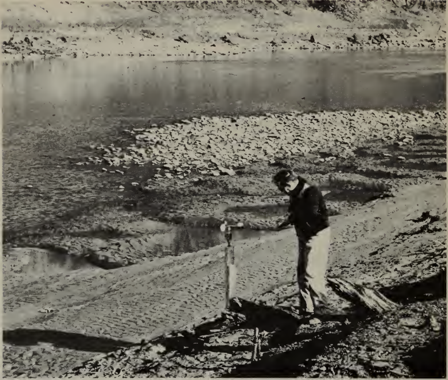
A Geological Survey scientist checks wind velocity in a thermal die-away study.
