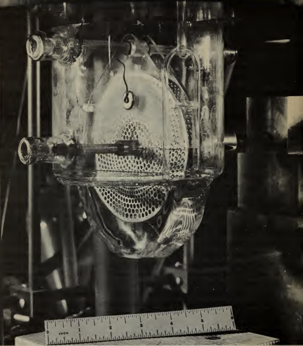
This experimental 4-inch diameter rotating-disc corona reactor is used for conversion of coal to liquids and gases.
