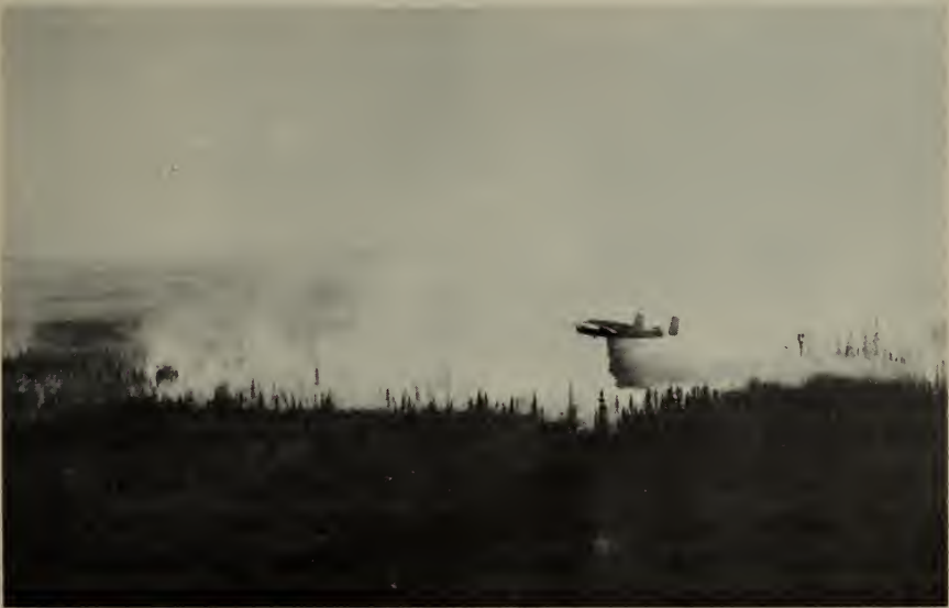
Dropping half of its 1,000-gallon load of fire-retarding borate on a forest fire near Bettles, Alaska, this converted B-25 bomber operates under contract with the Bureau of Land Management to help control forest fires in the far north.
