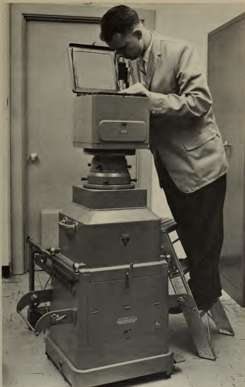
This new-model printer makes glass plate photographic transparencies with improved contrast for use in stereoscopic plotting instruments.
