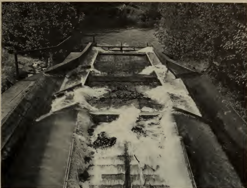
Incline-plane traps, such as this one on the Garlic River in Michigan, are used to capture and observe the downstream drift of sea lamprey ammocetes and developing sea lampreys.
