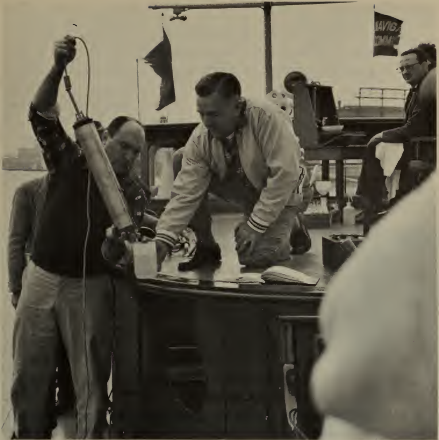
Water Resources Division chemists collect water samples from the Delaware River. Analytical equipment for determination of dissolved oxygen and specific conductance is in the background.—Courtesy City of Philadelphia.
