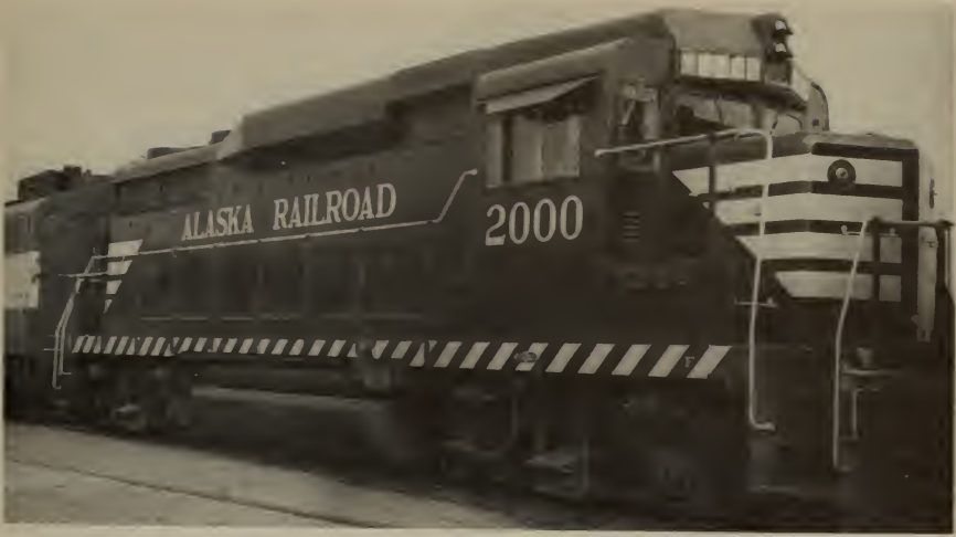
Placed in service during May 1963, this 2,250 horsepower diesel locomotive replaced another severely damaged by a snow slide in November 1961.
