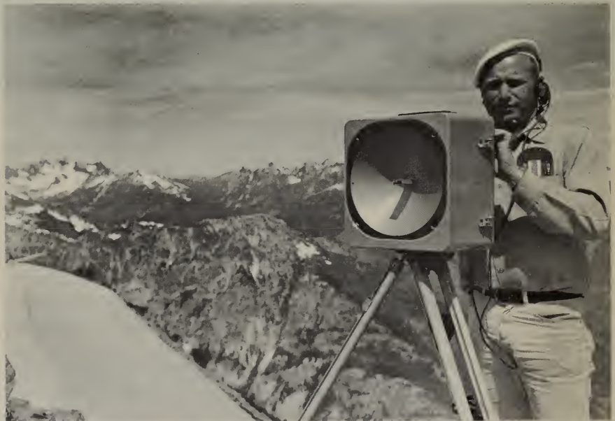
The latest electronic distance measuring equipment is used to obtain mapping control in rugged mountain terrain.
