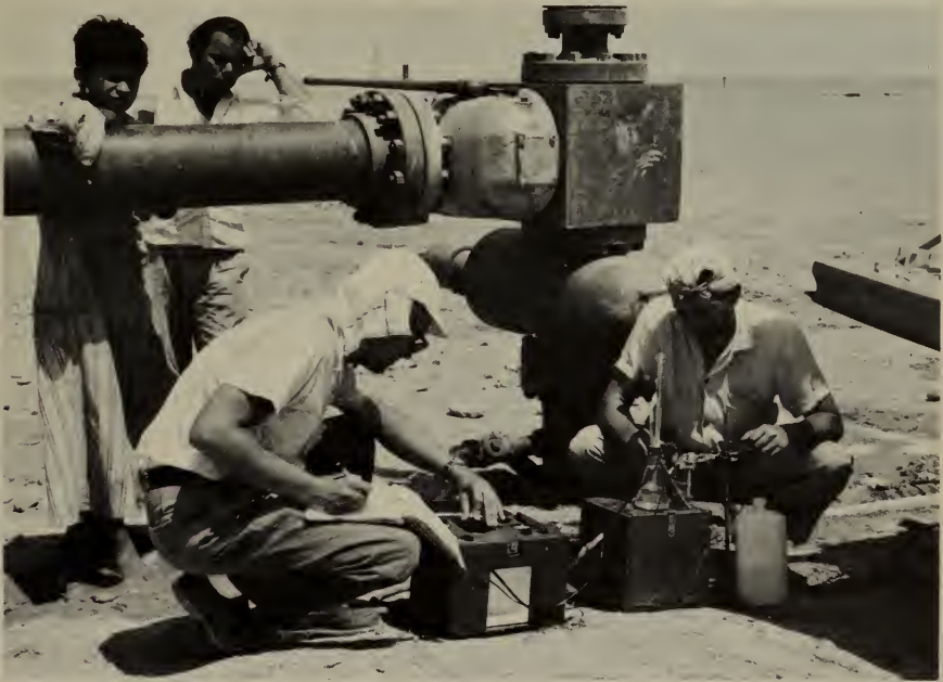
A Geological Survey engineer in Egypt conducts field tests on Gormashin well water for carbon dioxide at Kharga Oasis—part of the Department's program to assist other nations in natural resource development.
