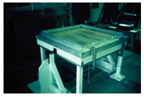
attached to the wood frame, with a lap joint in the middle, sealed with acoustical sealant, taped and stapled. The pressure box was equipped with a fan, a speed controller, an air flow meter and a pressure monitoring gage. A demonstration would consist of pressurising the box to simulate a wind pressure load on the construction assembly and the polyethylene film VB.
