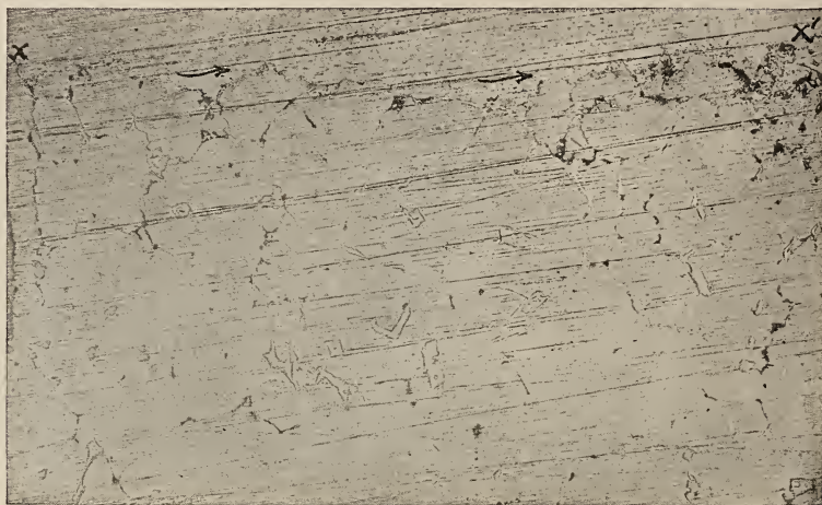
FIG. 28.—Microstructure of cast aluminum alloy showing the "path" of the fracture produced by a tensile stress. \times 100
