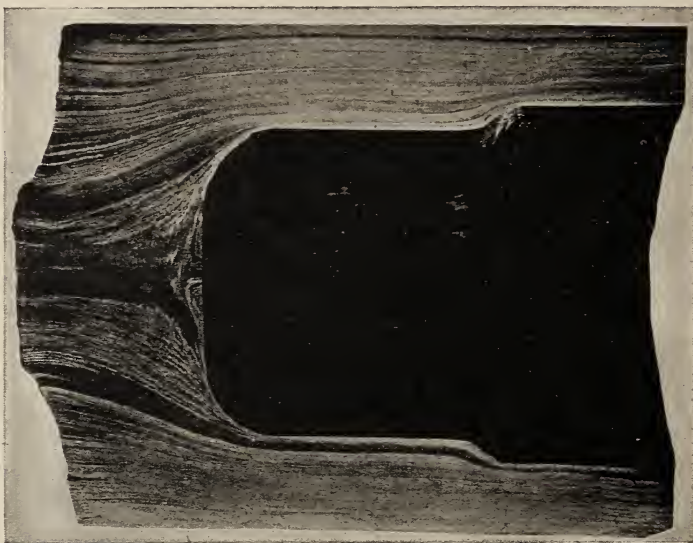
FIG. 5.—Macrostructure of forged steel (longitudinal section of the head of a shrapnel shell) revealed by etching with cupric chloride (Stead's reagent). \times 4/5
