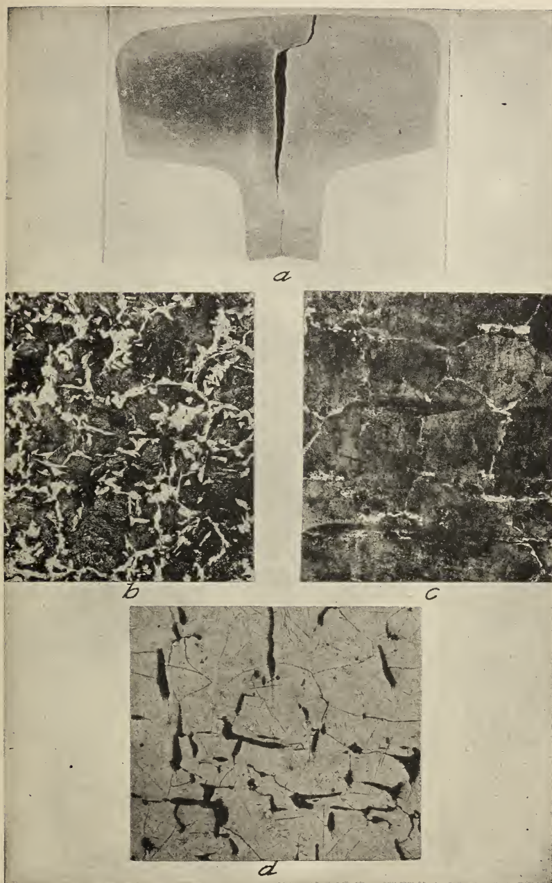
FIG. 16.—Variations in the microstructure of rail steel caused by segregation
