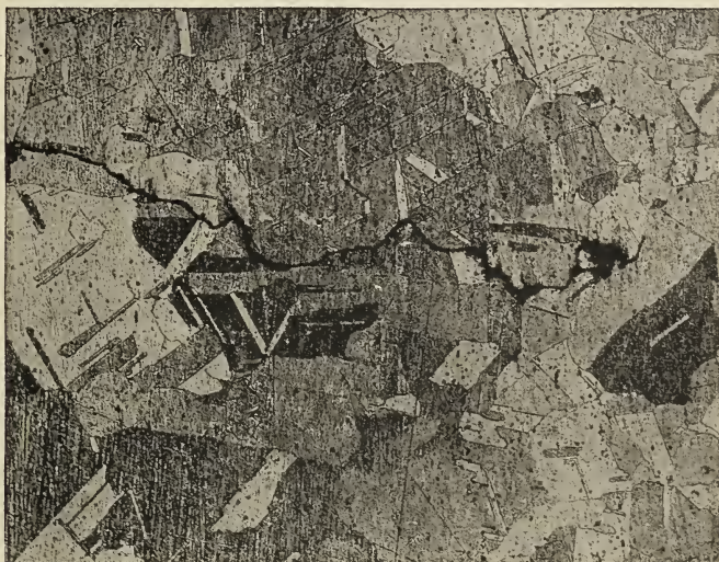
FIG. 46.—Microstructure of copper which was spoiled in annealing as a result of the nature of the surrounding atmosphere. \times 100
