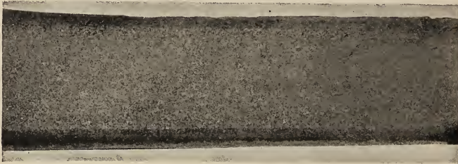
FIG. 58.—Macrostructure of a steel block showing surface changes caused by cutting the steel by means of the oxyacetylene flame. \times 1
