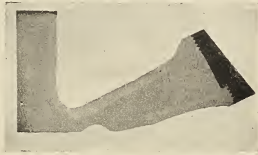
FIG. 70.—Macrostructure of a malleable-iron casting with which difficulties were experienced in the automatic machining to size. \times 1
