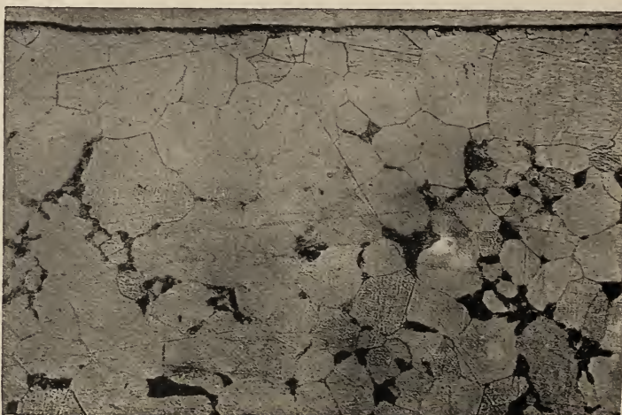
FIG. 51.—Microstructure of an iron-carbon alloy which was decarburized by heating in vacuo. \times 100
