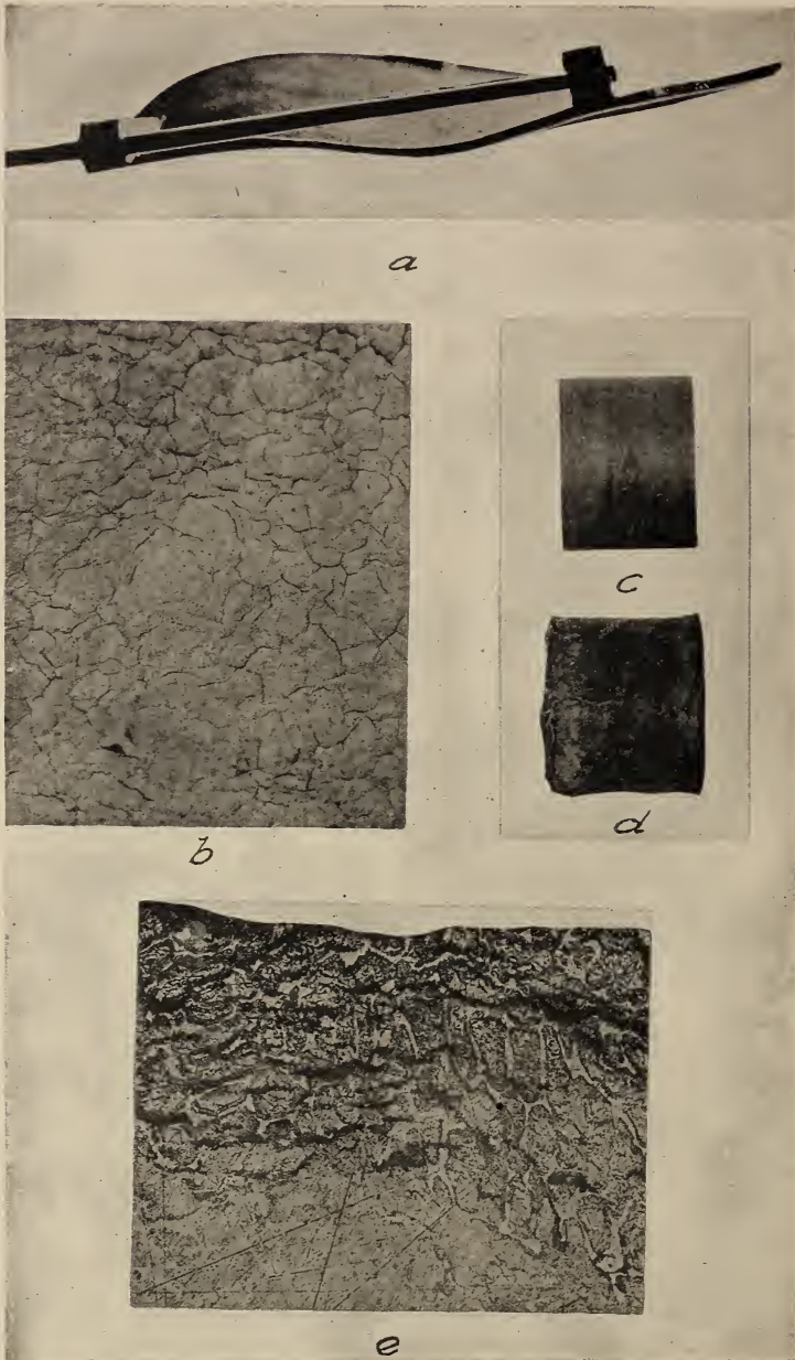
FIG. 64.—Appearance of certain aluminum alloys of high zinc content after deterioration
