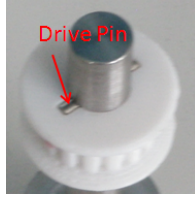
Figure 4.5: Drive pin mechanism used to replace previous set screws.
