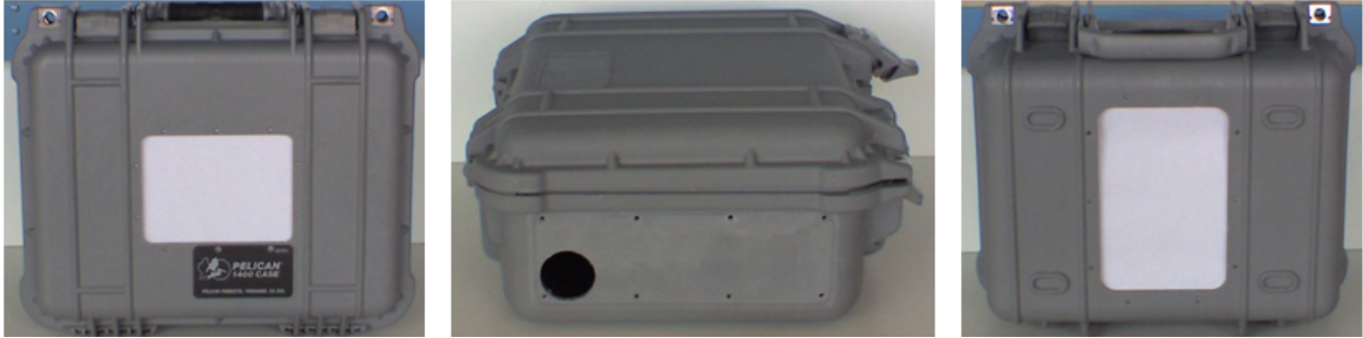
Figure 3.3: The Pelican case with cutouts for external modules.
