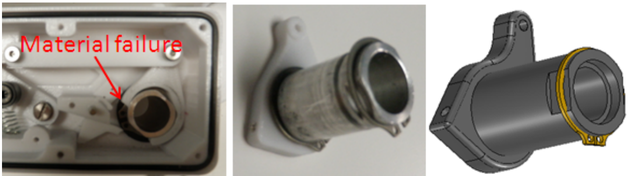
Figure 5.1: Left, Torque Arm failed, center, two-piece Torque Arm and Radial Arm Shaft, right, one-piece Torque Transmitting Radial Shaft.
