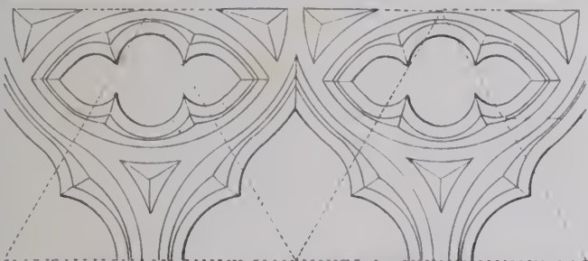
Tracery to W. side of Porch. Bradwell Ch. Essex. 1/2 nd scale.
