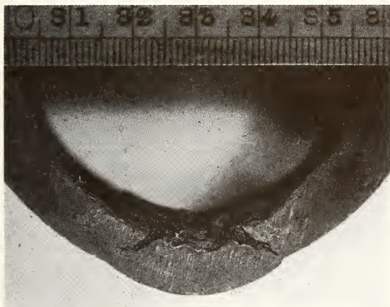
Fig. 2. Part-section through high-pressure boiler tube corroded from the inside almost to failure. The two radial fissures mark the extent of cracking of embrittled metal, but the outside of the tube has remained ductile and bulged rather than cracked.
