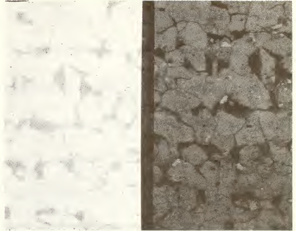
Fig. 6. Top view of the same area of a steel surface before and after magnetite formation. On the left the original polished steel surface has been conventionally etched to show the usual dark pearlite grains of the steel structure. On the right at the same magnification the view is of the protective magnetite formed on that same area of steel. The pearlite grains, still averaging 10\ \mu\text{m} in size but now only ghosts have clearly been undisturbed during their oxidation to magnetite, showing that the magnetite layer forms without significant stress.
