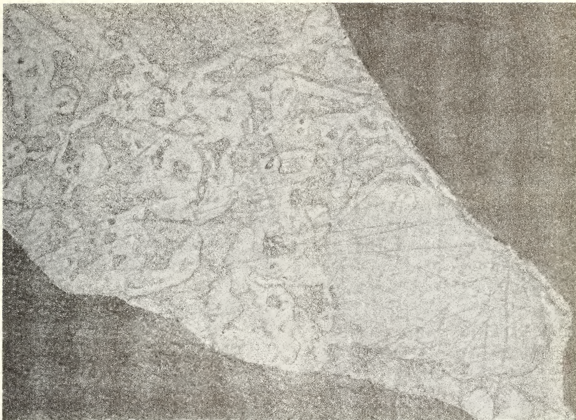
Fig. 2. Reaction rim of maldonite (light grey) surrounding and filling corrosion voids in gold in an outer bismuth matrix which has reacted with the gold by solid-state diffusion. Reflected light photomicrograph, phase contrast enhanced electronically. Area of specimen shown 1.5 mm x 1.0 mm.
