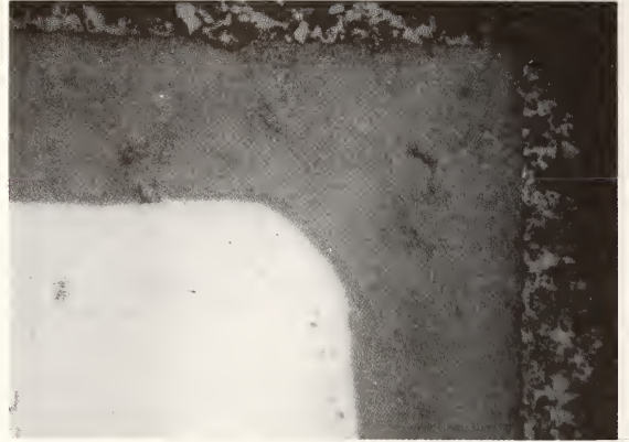
Fig. 7. At a sharp corner the original profile of the steel is retained as protective magnetite, but the acceleration of the oxidation there makes the steel/magnetite interface rounded.
