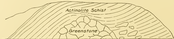
FIG. 17.—Intrusive greenstone in grünerite-magnetite-schist, from near center of sec. 12, T. 47 N., R. 29 W.
