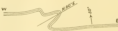
FIG. 23.—Horizontal plan of one of the minor pitching isoclinal folds in the grünerite magnetite-schist.
