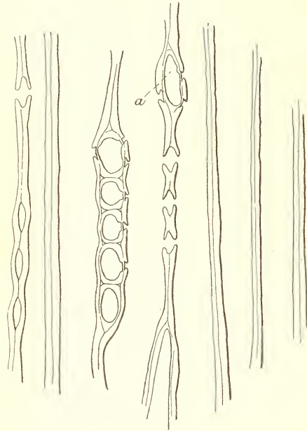
FIG. 5.—Tangential section of mature wood: a , a medullary ray of but one cell row. These are quite common—greatly enlarged.
