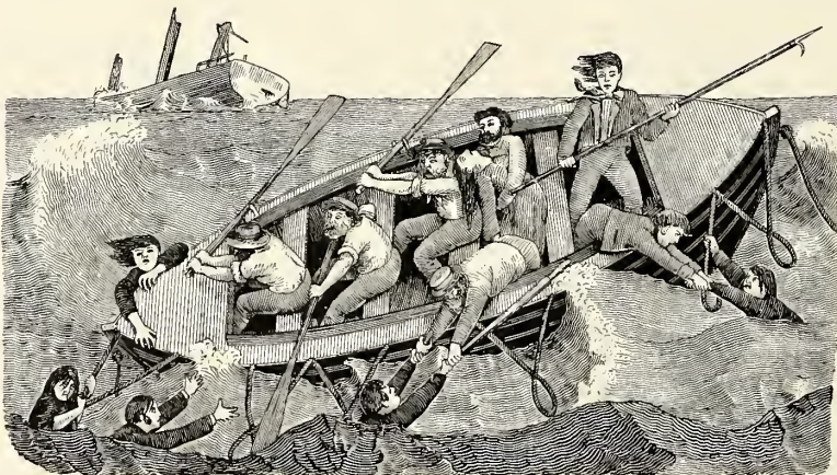
OLD ENGRAVING SHOWING THE FIRST LIFE-BOAT. THIS BOAT, MADE OF WOOD, AND LINED WITH CORK, WAS USED AT A WRECK IN 1817.
