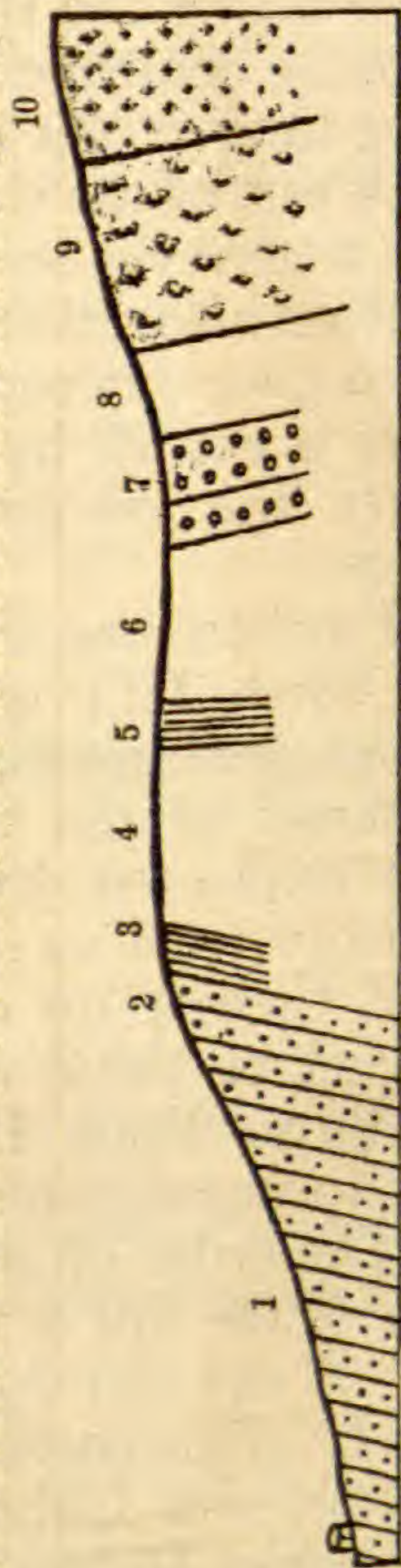
Fig. 5.—Section southerly from Fitch's house. 1, Diabase; 2, Quartz; 3, Slates; 4, Fossils in limestone; 5, Slates; 6, Limestone; 7, Conglomerate; 8, Siliceous limestone; 9, Hornblende; 10, Sandstone.
