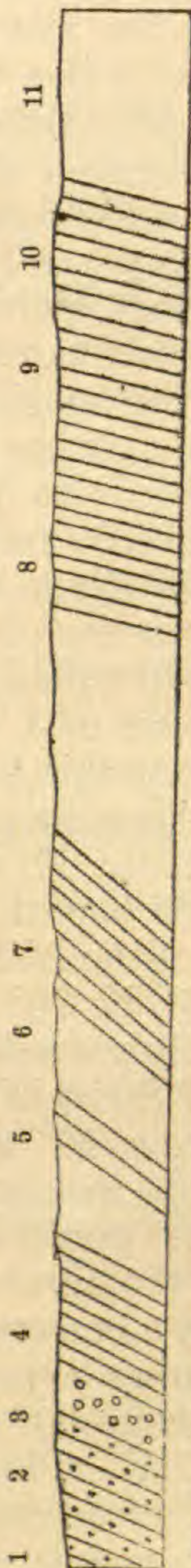
Fig. 11.—Section through Swift Water village. 1, Starch mill; 2, Lisbon group; 3, Micaceous conglomerate; 4, Slate; 5, Gneissic; 6, Mica schist; 7, Swift Water village, chloritic; 8, Mica schist; 9, Hornblende schist; 10, Micaceous quartzites; 11, Gneiss.
