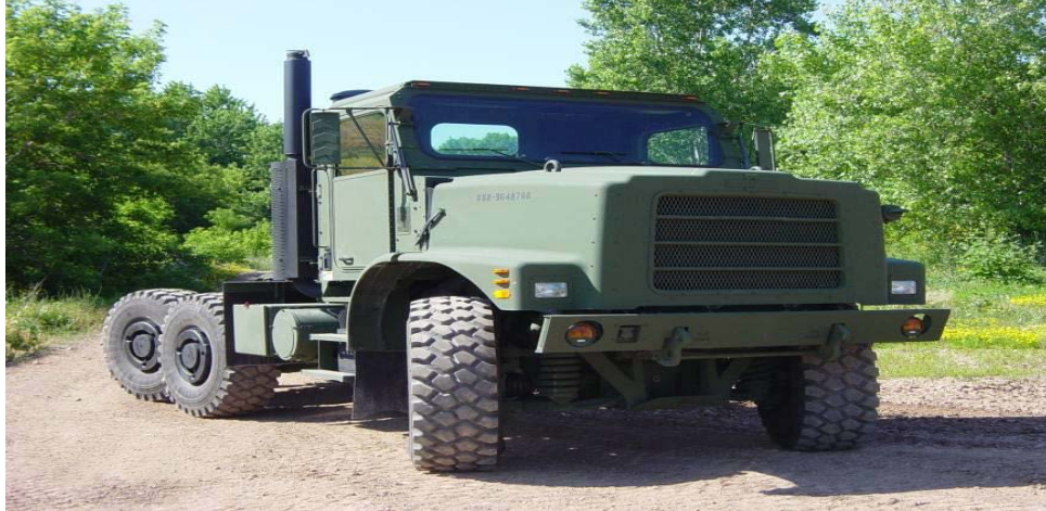
Figure 1. MK31/MK31A1 Tractor: Prime Mover for MK970/AMK970 5,000 Gallon Refueler. Source: Program Executive Officer, Land Systems (PEO LS) Marine Corps (2016).
