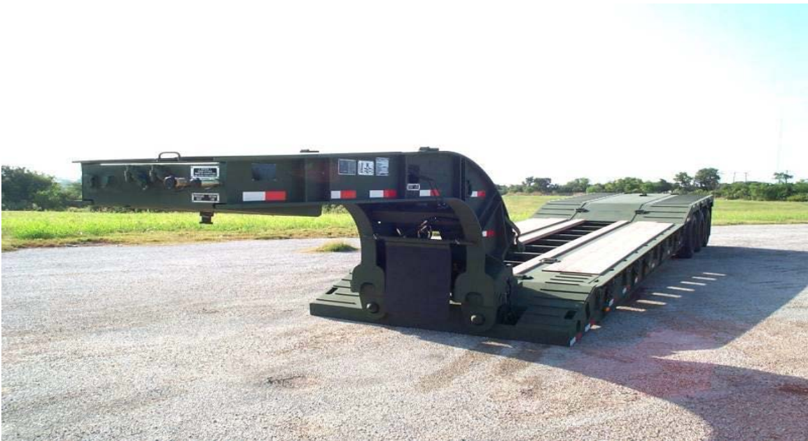
Figure 13. M870A2E1 Medium Heavy Equipment Transporter (MHET). Used in conjunction with MKR16. Source: POE LS Marine Corps (2016).
