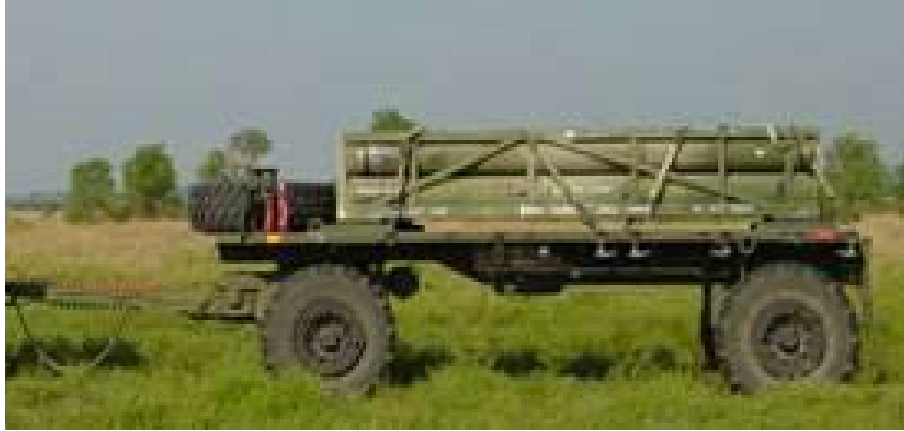
Figure 5. Medium Tactical Vehicle Replacement (MTVR) MK38 HIMARS Re-Supply Trailer. Source: POE LS Marine Corps (2016).
