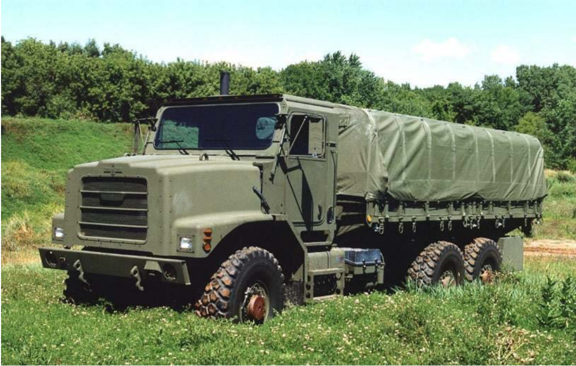
Figure 3. MK28/MK28A1: Large Capacity Troop and Medium Cargo Carrier. Source: PEO LS Marine Corps (2016).
