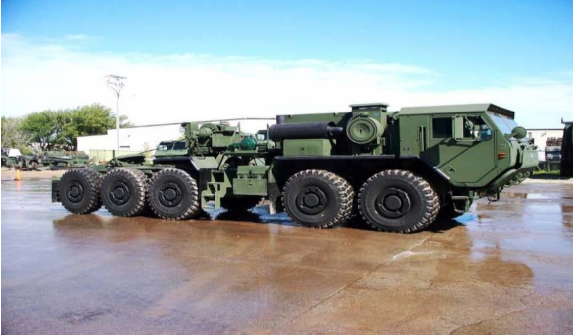
Figure 12. MKR16/AMKR16 Tractor. Transports Heavy Cargo when Trailer Attached. Source: POE LS Marine Corps (2016).
