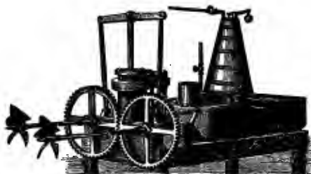
FIG. 84.—Engine, Boiler, and Screw-Propellers used by Stevens, 1804.
