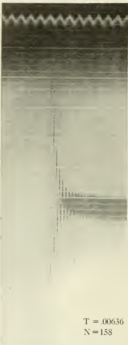
FIGURE 2. Vibration tests of manometer. Upper record, tuning fork .02 second.
