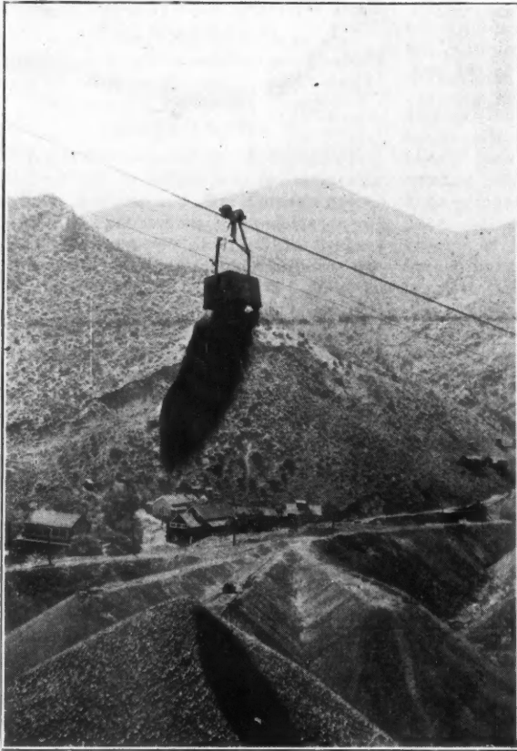
NEW IDRIA QUICKSILVER MINING CO., IN CALIFORNIA, DELIVERS RED HOT CALCINES TO DUMP BY AERIAL TRAMWAY
