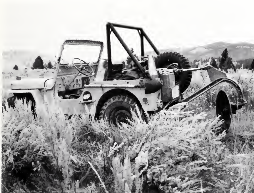
Figure 2—Plow unit in operation in a sagebrush area.
