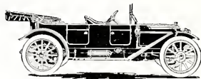
Marathon Model L-30 Touring Car 116-in. Wheelbase, 34 x 3½ Tires, Full 30 H. P. Complete Equipment, $1,200
